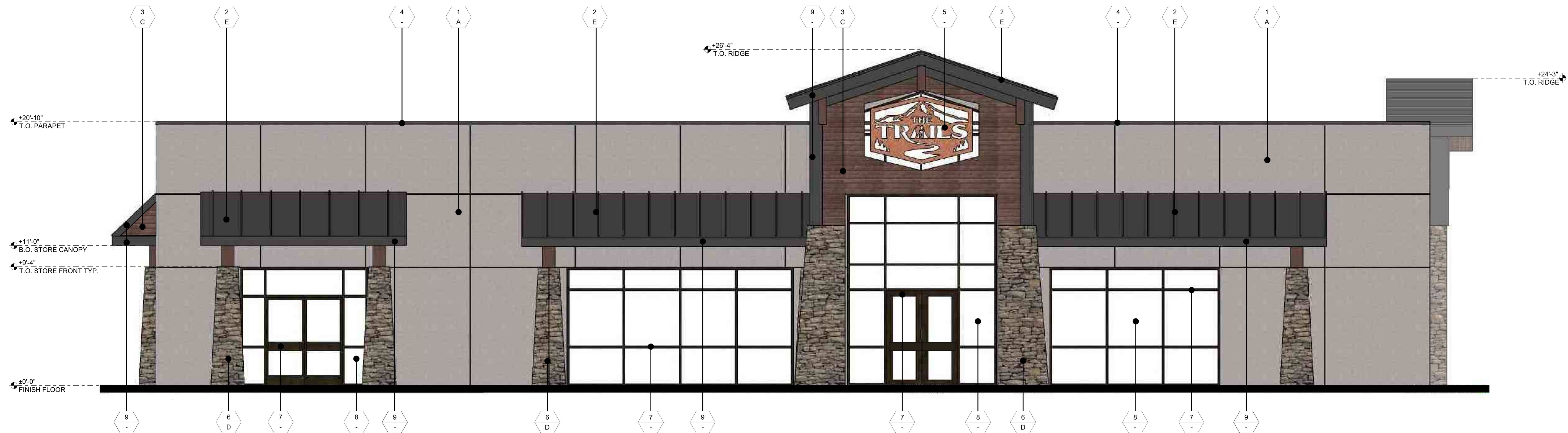
1 EXTERIOR ELEVATION - WEST 1/4" = 1'-0"
