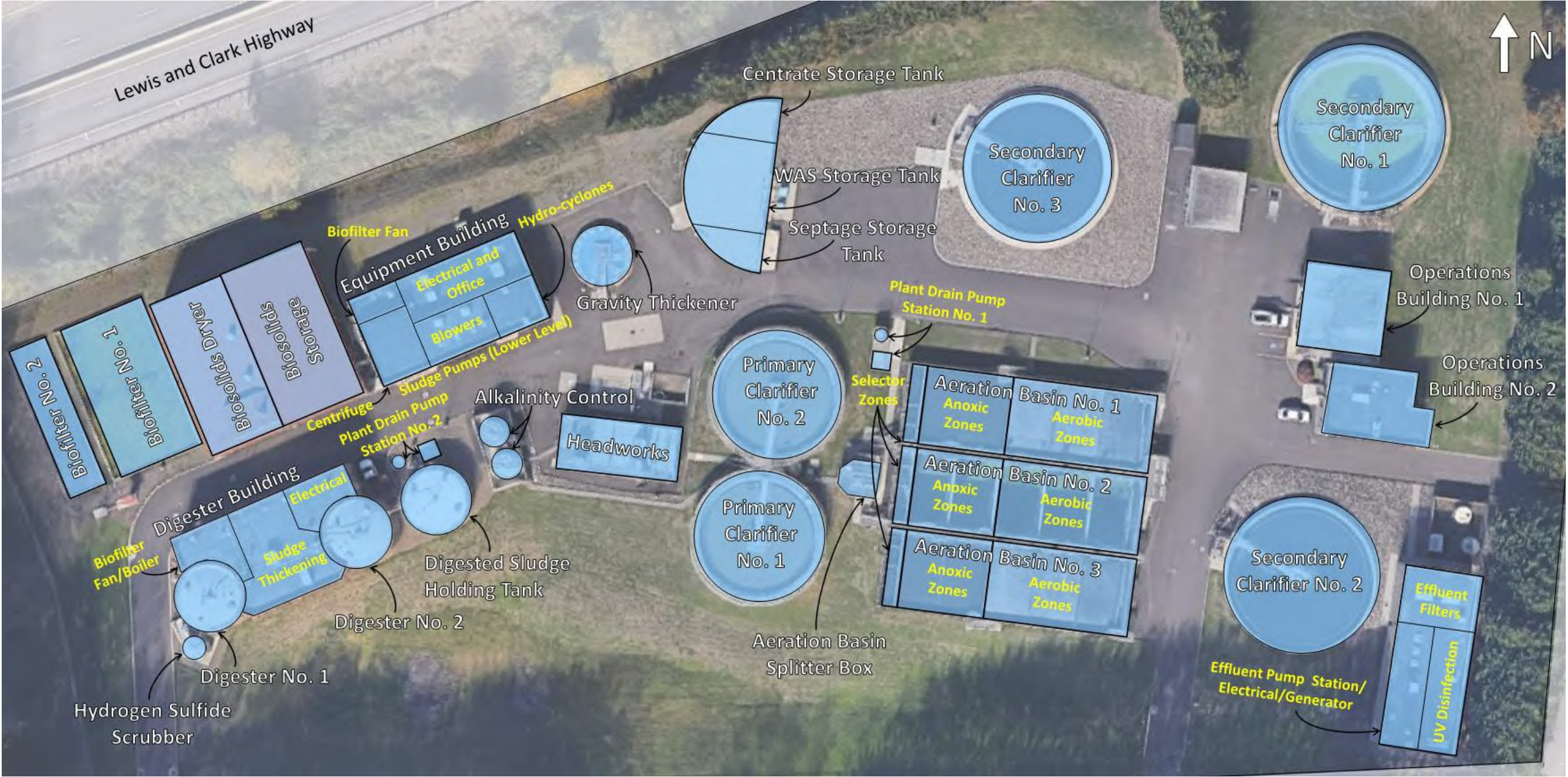
Figure 4.5 WWTf Aerial Image with Site Plan
