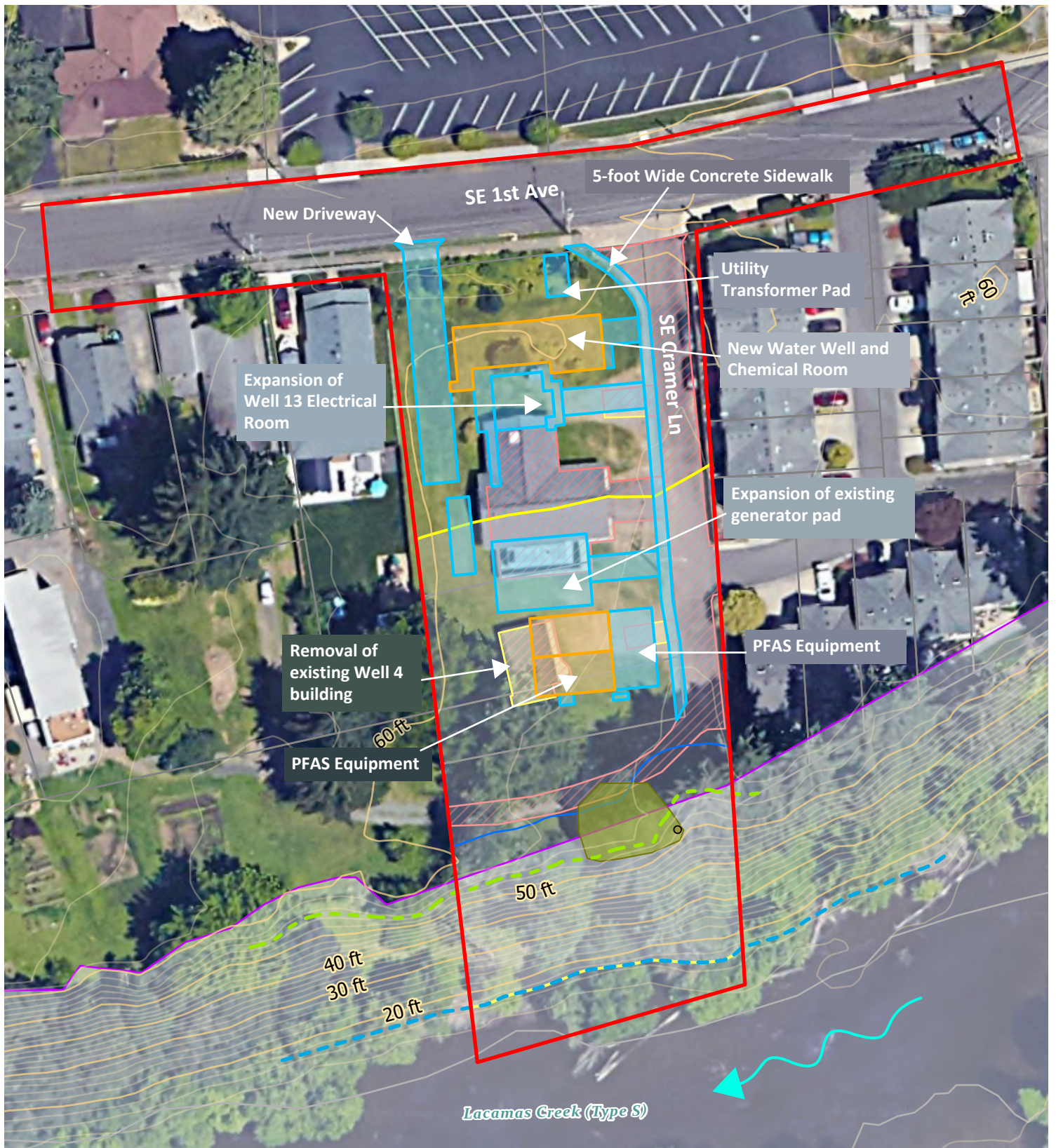
Figure 3. Proposed Conditions Camas Well 13 PFAS Treatment Design
