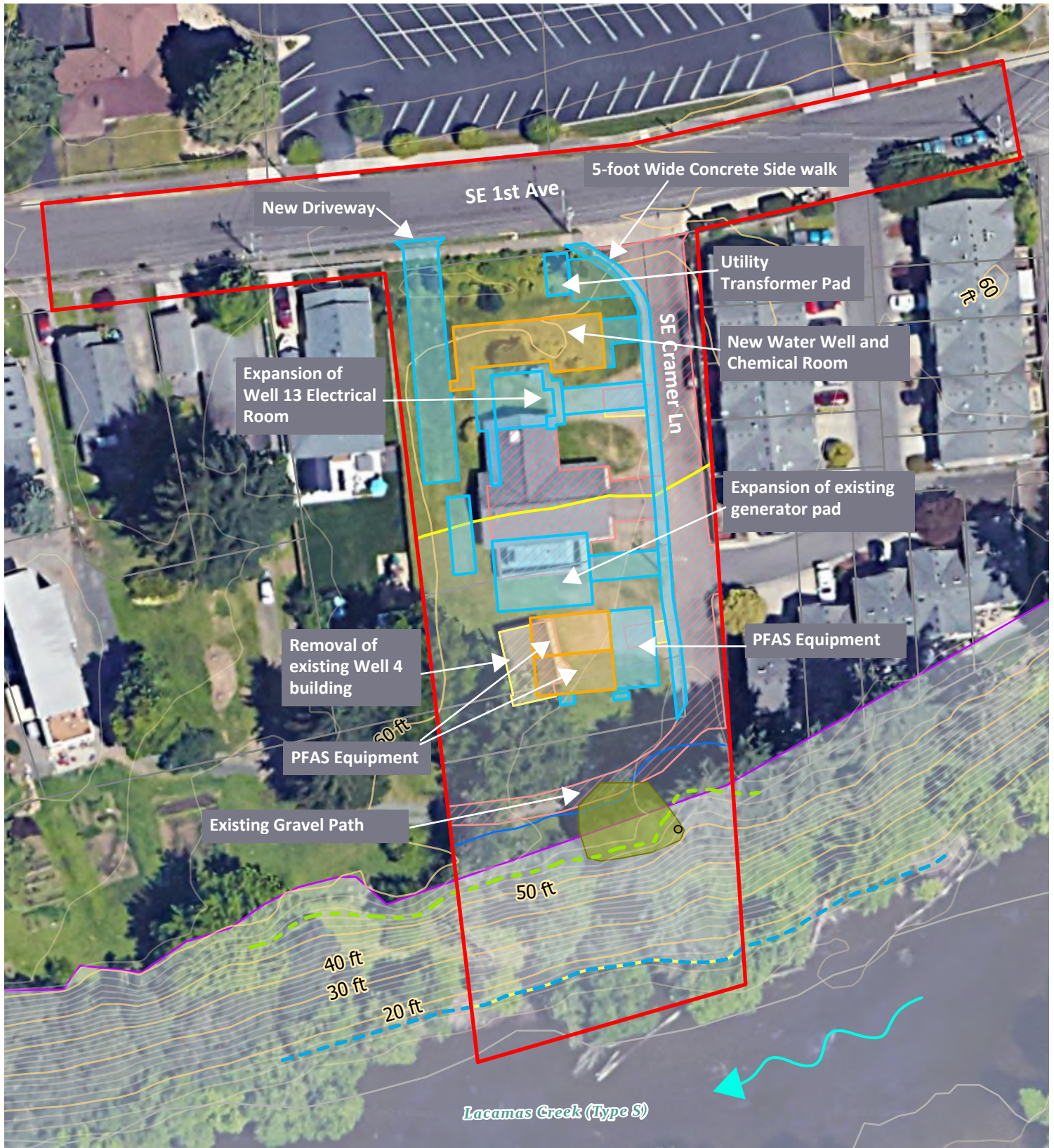
Figure 3. Proposed Conditions Camas Well 13 PFAS Treatment Design
