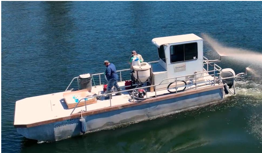
Figure 2: Close-up of Boat Spray Application on Kitsap Lake
