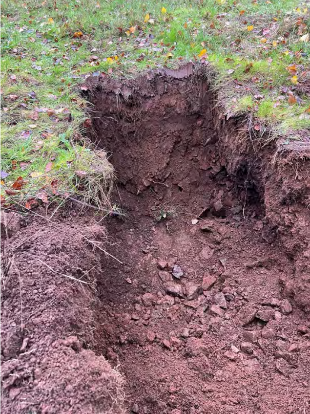
I-1. Bedrock @ 2.5 ft. bgs
