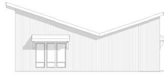
Main Right Elevation 1/8" = 1'-0"
