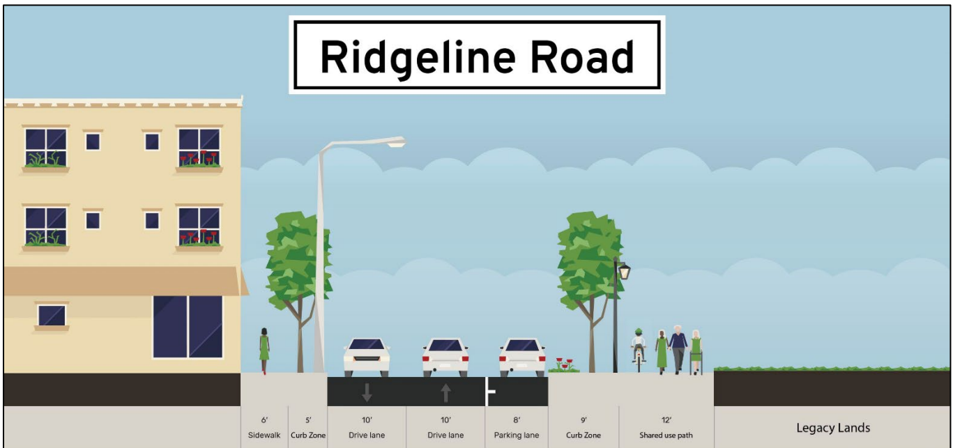
Figure 15. Ridgeline Road Cross Section
