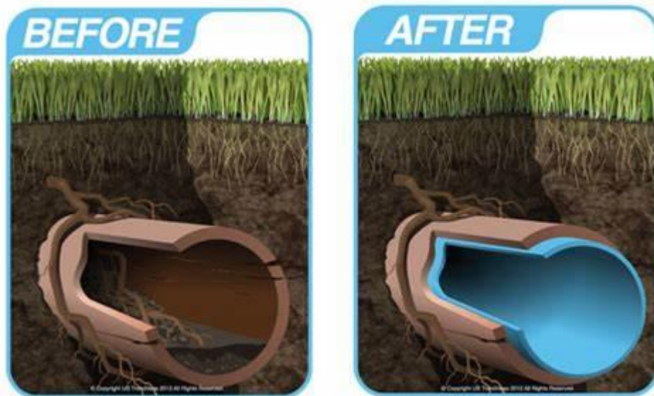
Figure 2. Illustration of before and after CIPP
