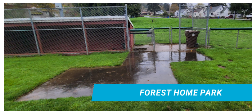
Poor drainage and limited sidewalk connections near the dugouts at Forest Home Park affect accessibility, user safety, and overall field usability.
