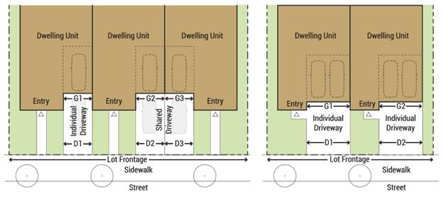
(G1+G2+G3)/Lot Frontage must be no more than 60% (D1+D2+D3) must not exceed 64 feet per frontage Individual driveway width (D1) and shared driveway widths (D2+D3) shall not exceed 20 feet
