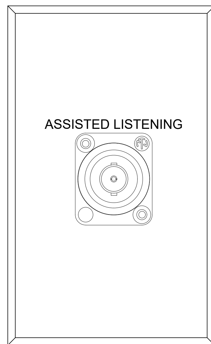
1 ASSISTED LISTENING (WA) PLATE DETAIL Scale: NTS
