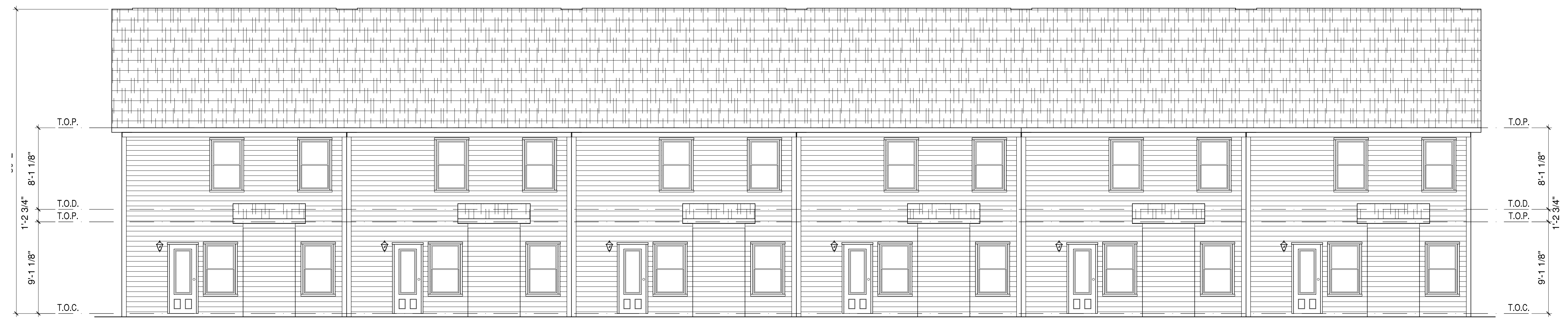
3 BUILDING B - BACK ELEVATION - "STYLE D" SCALE: 3/16"=1'-0"
