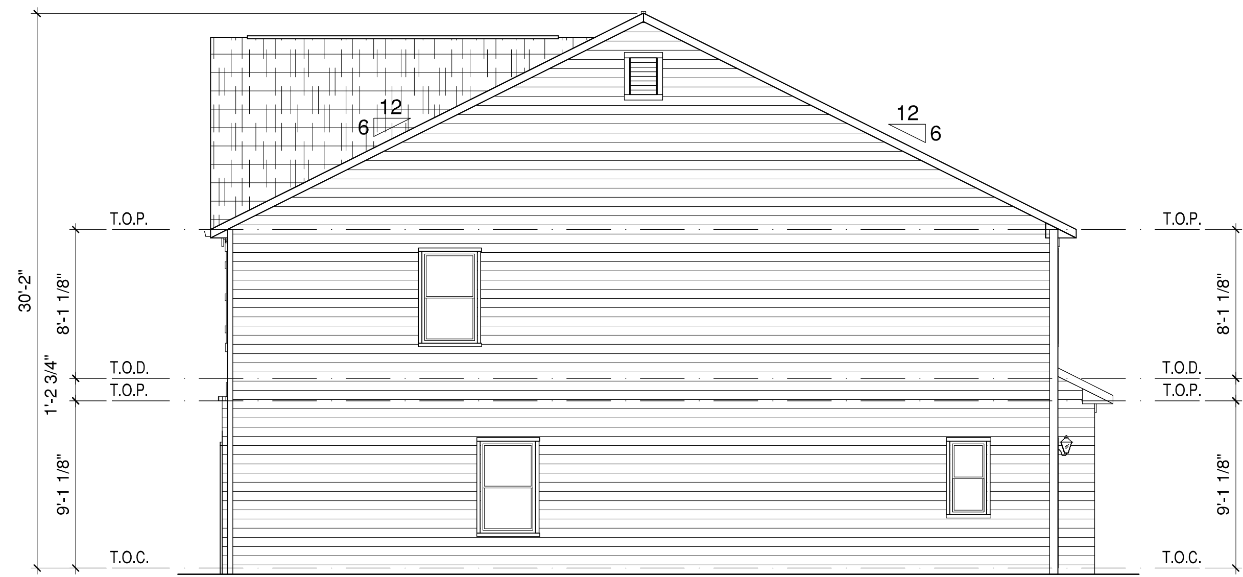
2 BUILDING A - END ELEVATION - "STYLE A" SCALE: 3/16"=1'-0"
