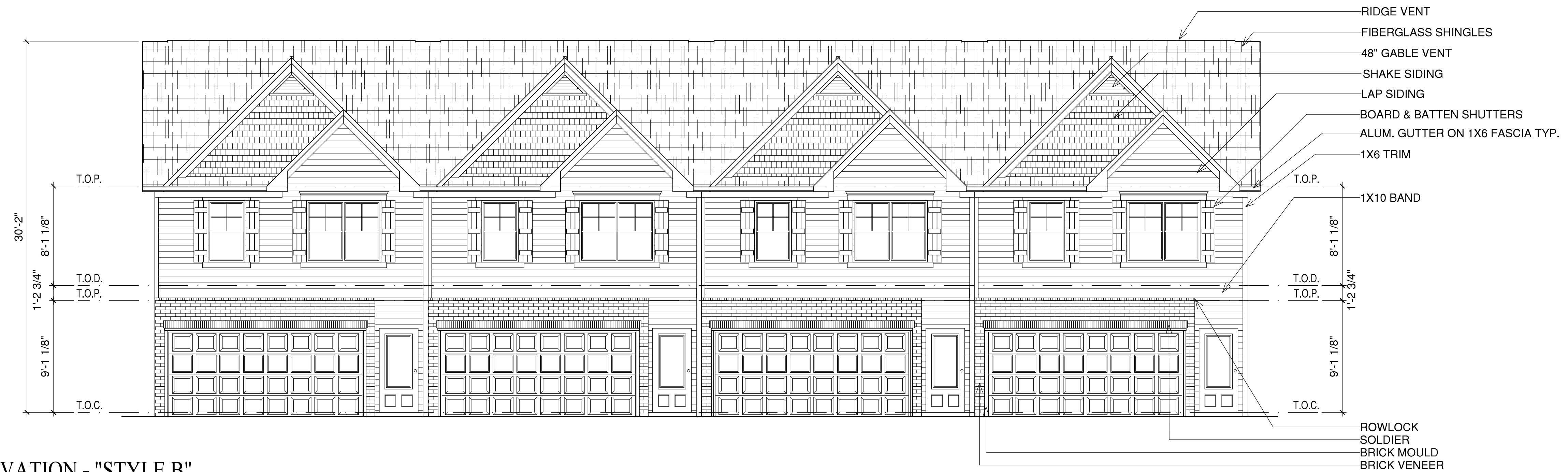
1 BUILDING A - FRONT ELEVATION - "STYLE B" SCALE: 3/16"=1'-0"
