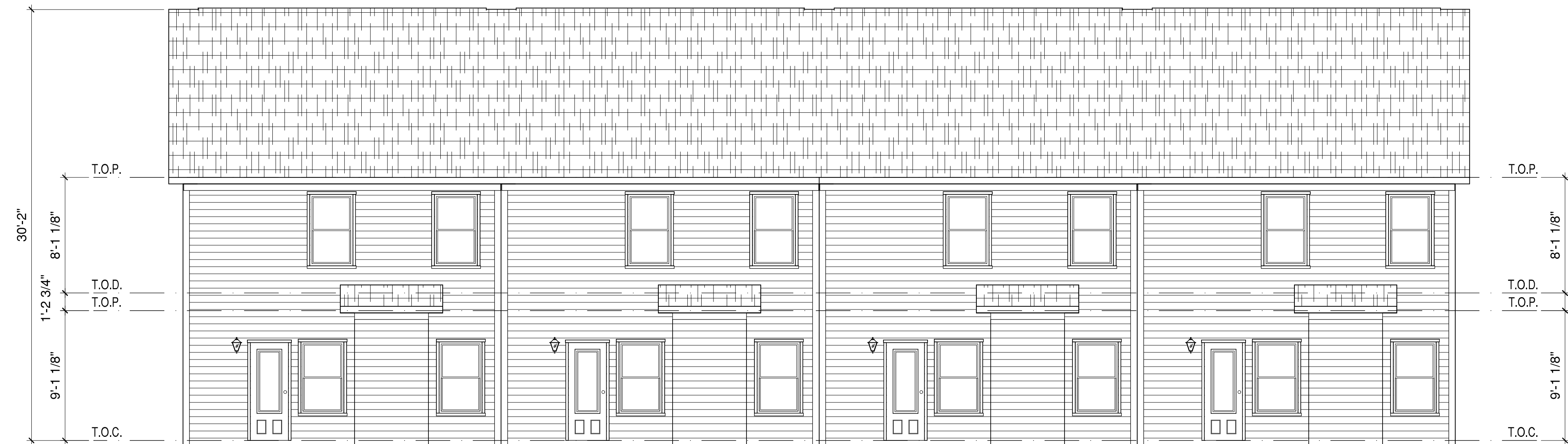
3 BUILDING A - BACK ELEVATION - "STYLE A" SCALE: 3/16"=1'-0"
