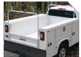
OVERHEAD LADDER RACK
