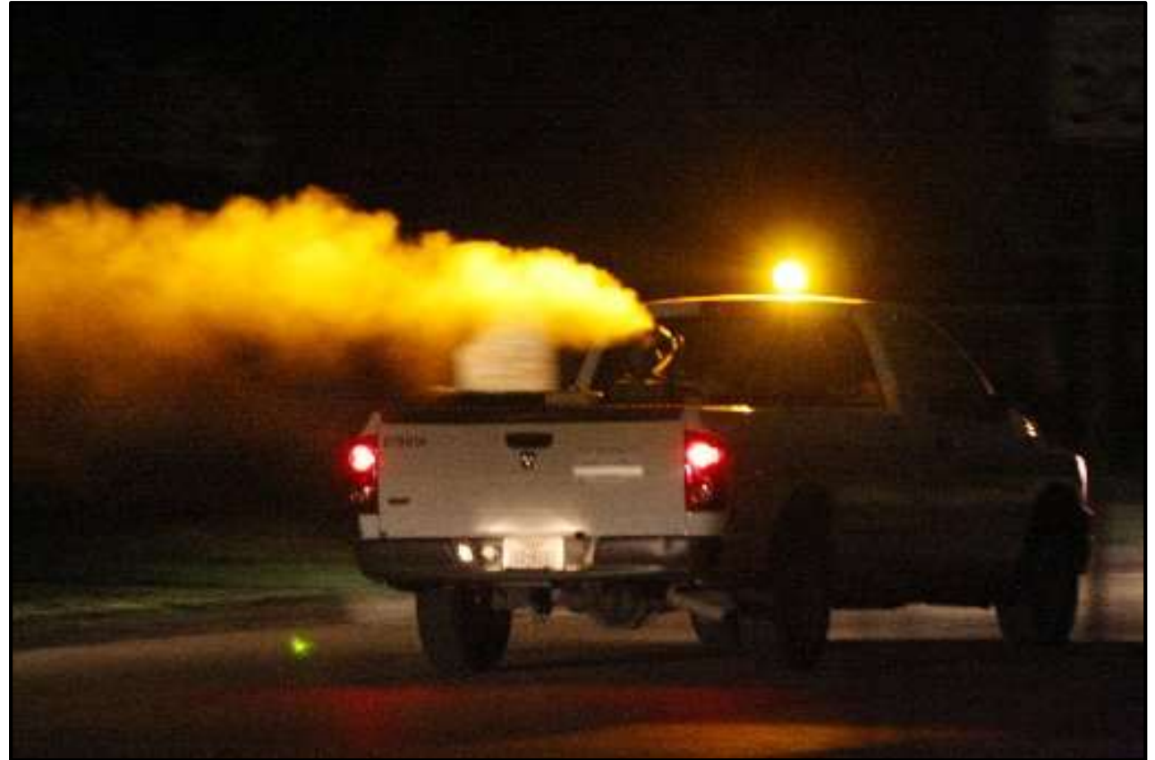
Truck conducting ground-based Ultra Low Volume fogging
