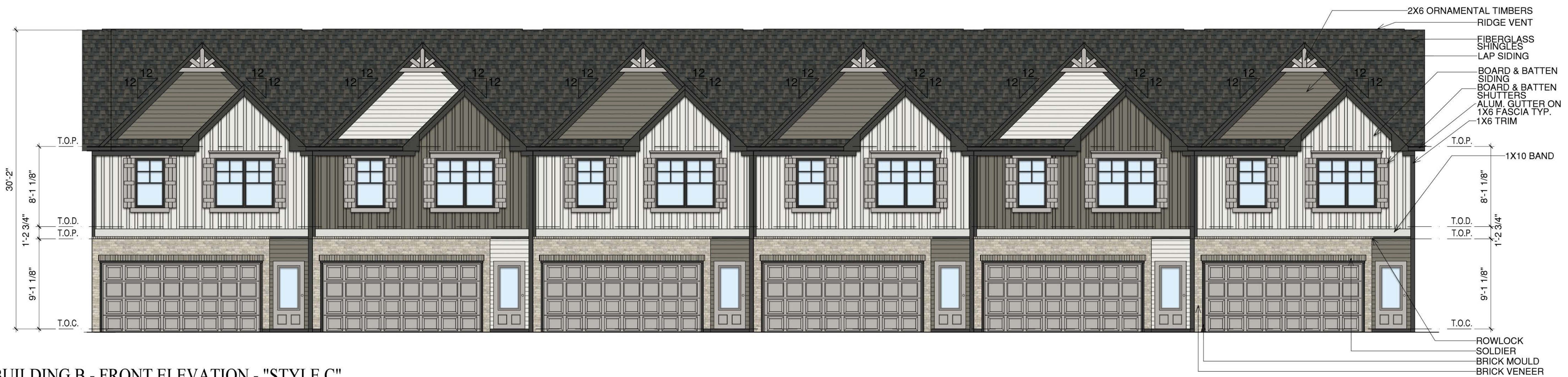
1 BUILDING B - FRONT ELEVATION - "STYLE C" SCALE: 3/16"=1'-0"
