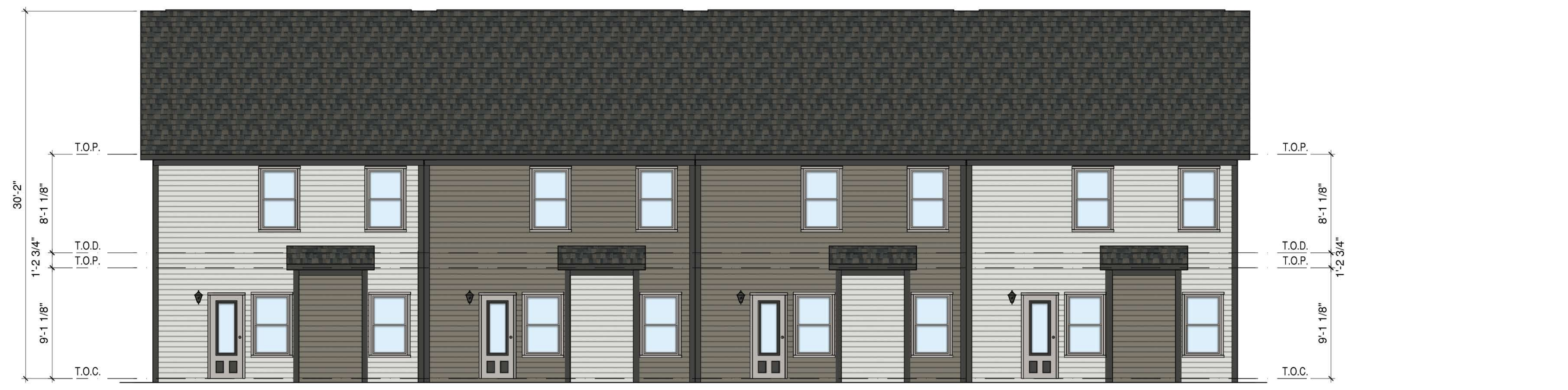
3 BUILDING A - BACK ELEVATION - "STYLE B" SCALE: 3/16"=1'-0"
