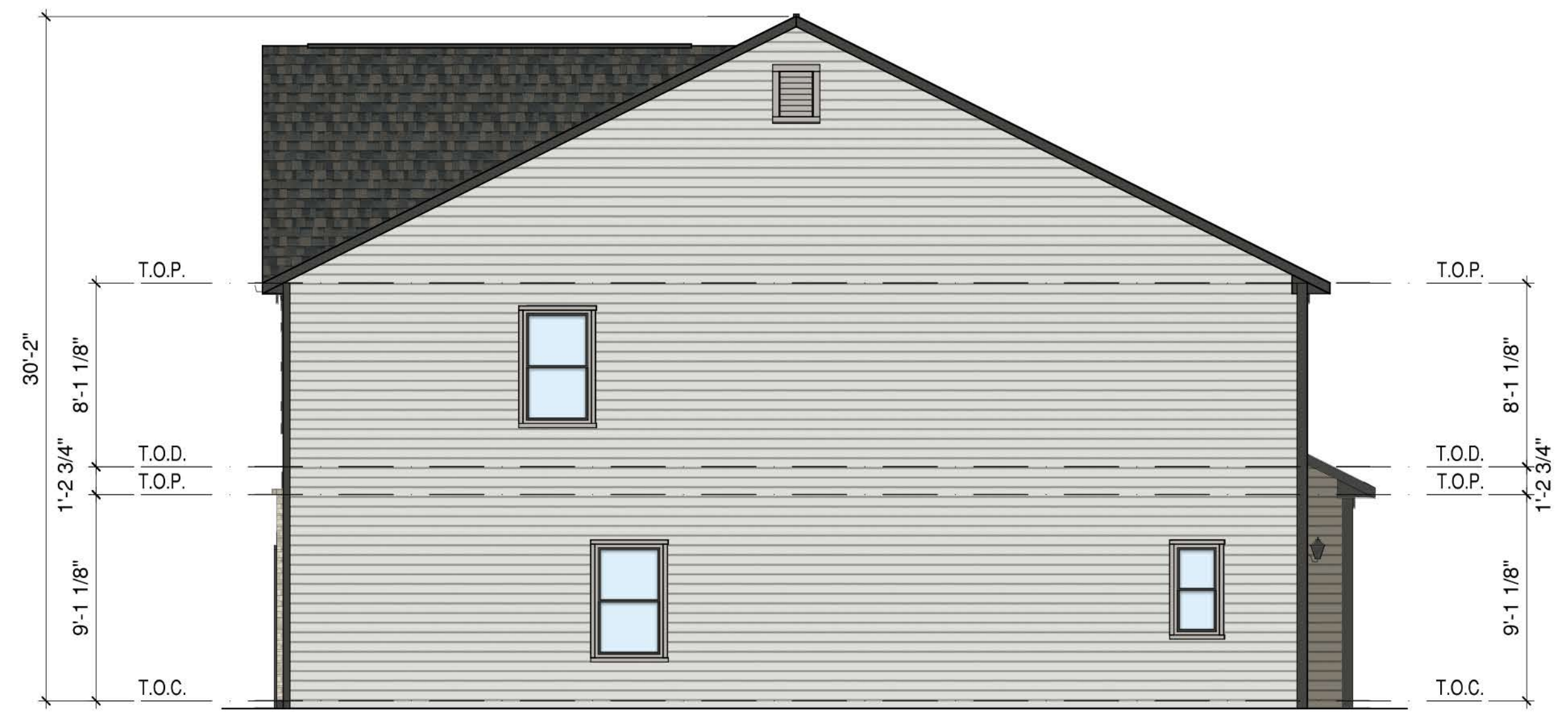
2 BUILDING A - END ELEVATION - "STYLE B" SCALE: 3/16"=1'-0"
