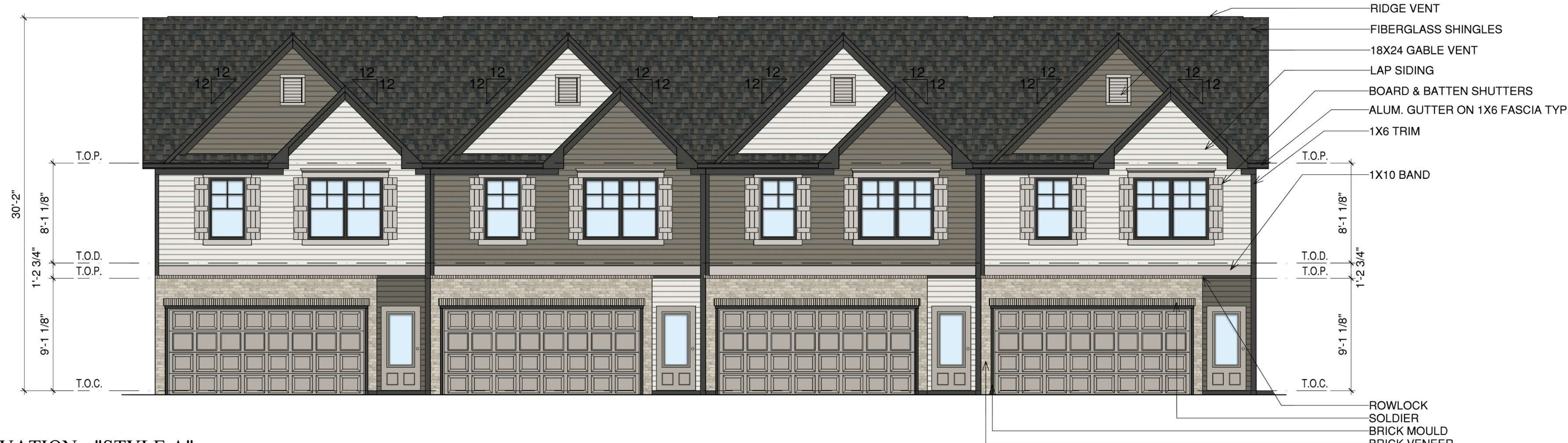
1 BUILDING A - FRONT ELEVATION - "STYLE A" SCALE: 3/16"=1'-0"
