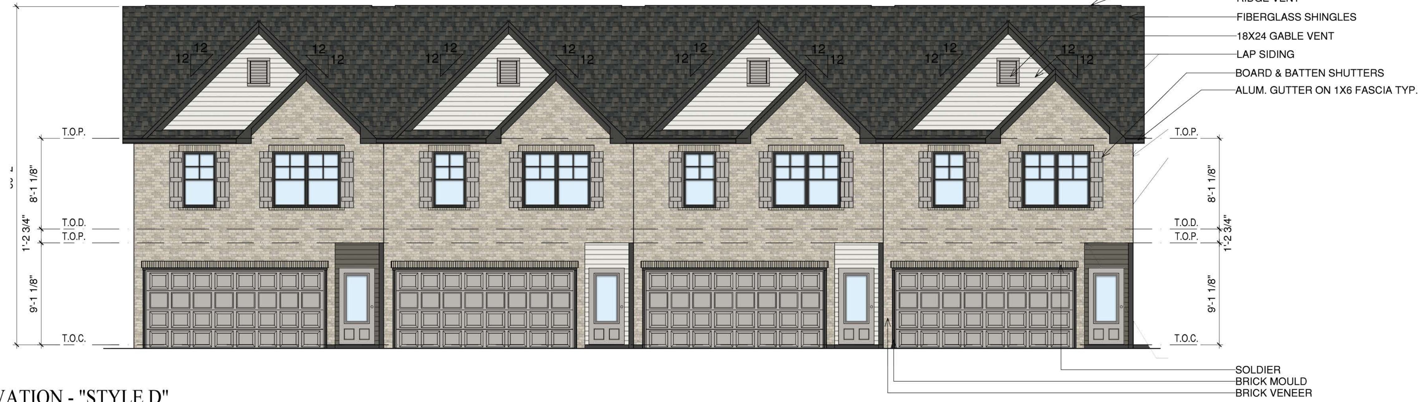
1 BUILDING A - FRONT ELEVATION - "STYLE D" SCALE: 1/8"=1'-0"
