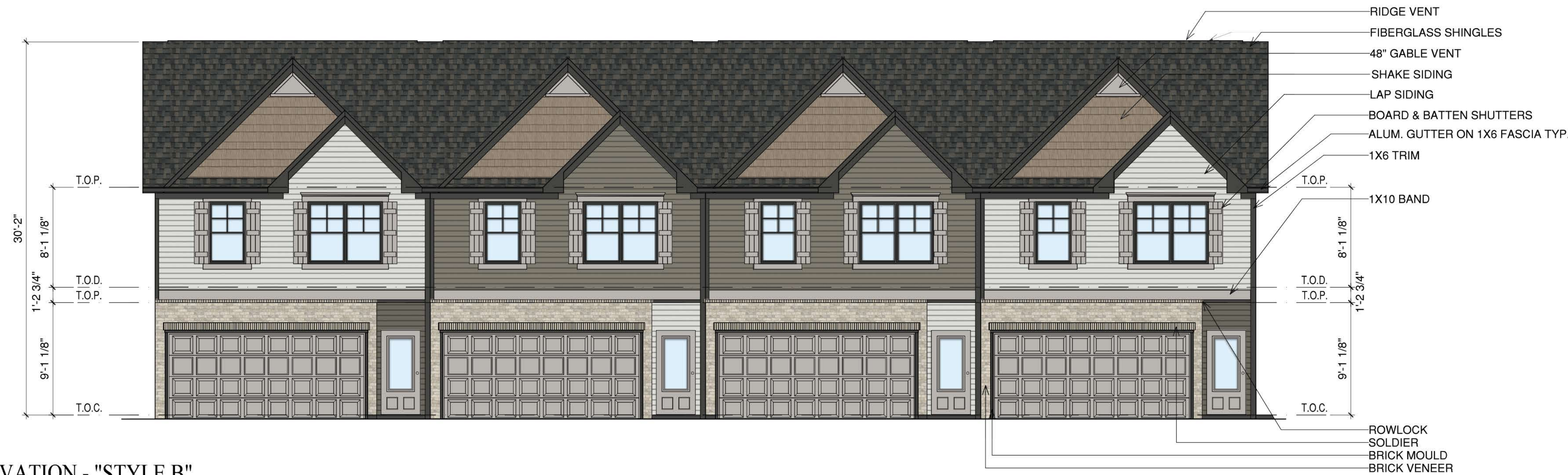
1 BUILDING A - FRONT ELEVATION - "STYLE B" SCALE: 3/16"=1'-0"
