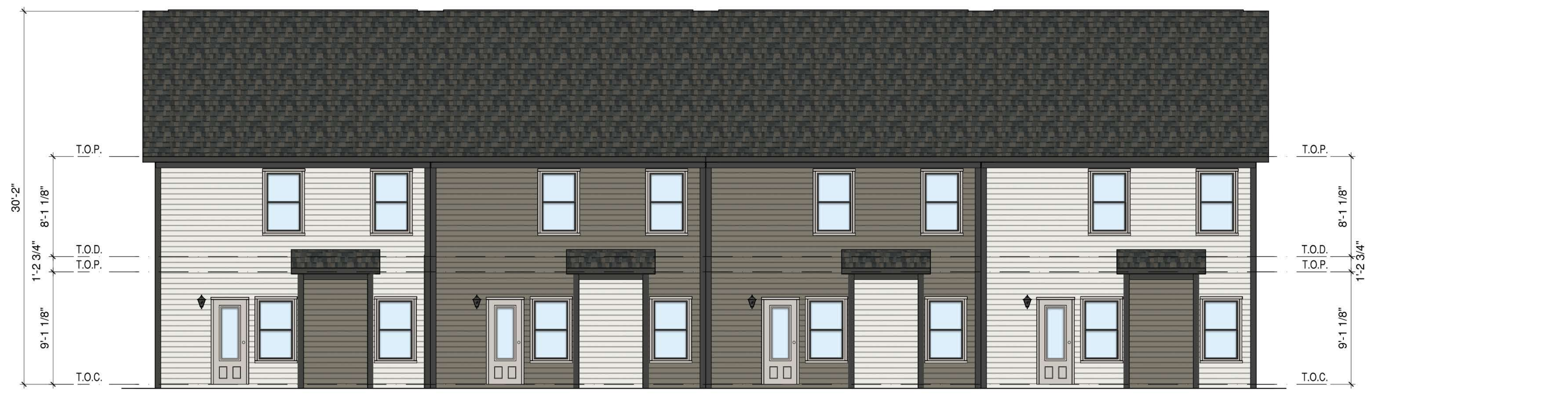
3 BUILDING A - BACK ELEVATION - "STYLE A" SCALE: 3/16"=1'-0"
