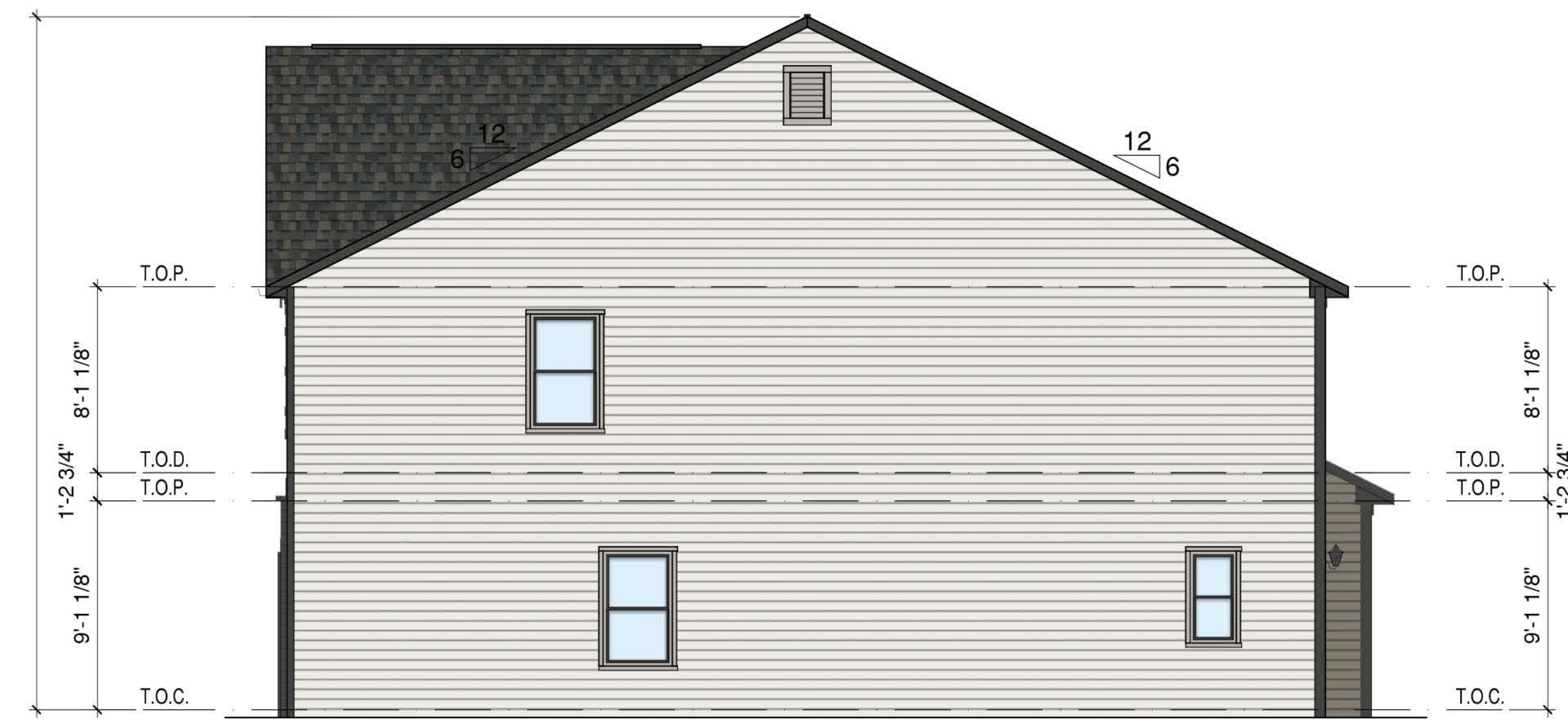
2 BUILDING B - END ELEVATION - "STYLE A" SCALE: 3/16"=1'-0"
