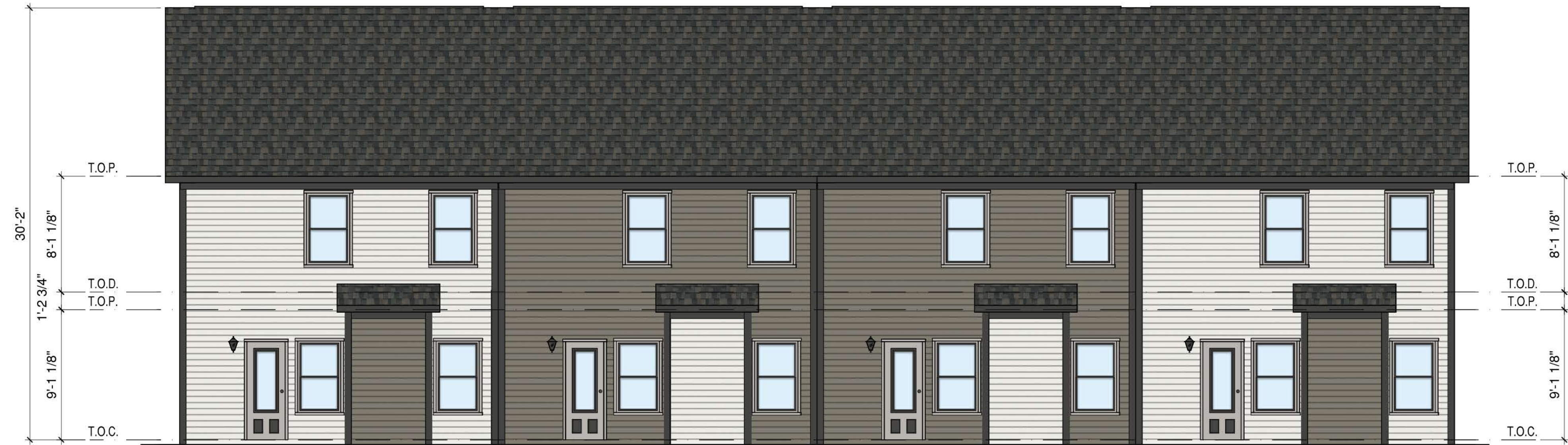
3 BUILDING A - BACK ELEVATION - "STYLE D" SCALE: 1/8"=1'-0"
