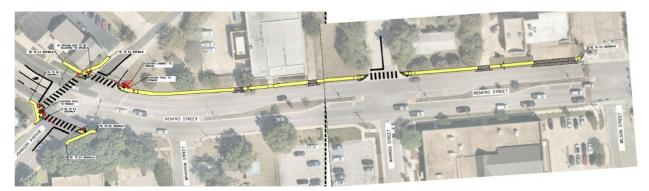
The project will increase pedestrian mobility in the District by providing sidewalks along the north side of W Renfro St from N Wilson St to NE Johnson Ave and along the intersection of Renfro and Johnson. The project will include crosswalks, ramps, and signal improvements to make the connection ADA compliant.
