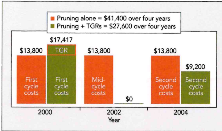
The use of TGRs results in a 35% cost reduction over four years
