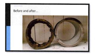
This picture shows the interior of a cast iron pipe, before and after being cleaned, and the cement-mortar lining applied. (Note: New ductile iron pipe that is currently being installed in our system, comes with a factory installed cement-mortar lining.)
