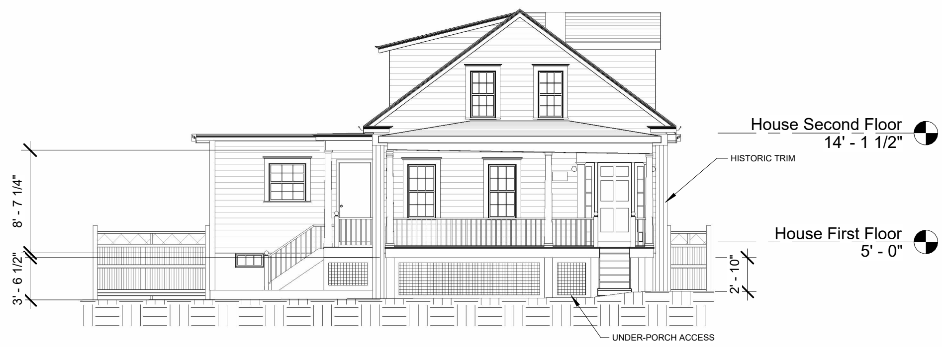
① Existing South Elevation 1/8" = 1'-0"
