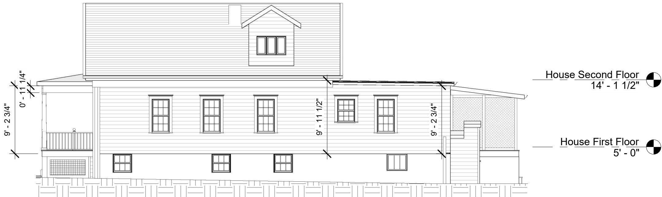
2 Existing East Elevation 1/8" = 1'-0"
