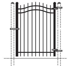
ATF Panels are 94" actual length • All gates listed are single swing and welded with 1-1/4" x 16 ga Gate Ends and Caps • Hinges sold separately
