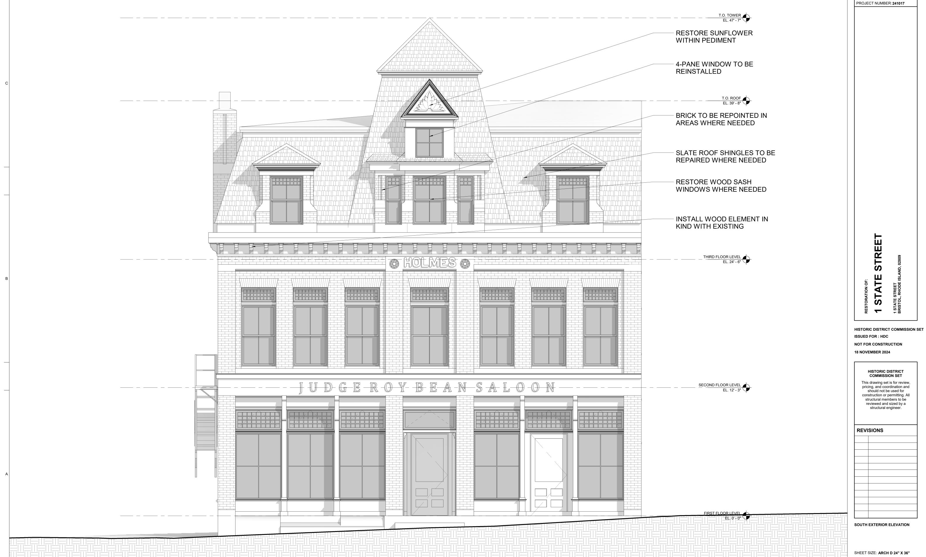
A5 PROPOSED SOUTH EXTERIOR ELEVATION
