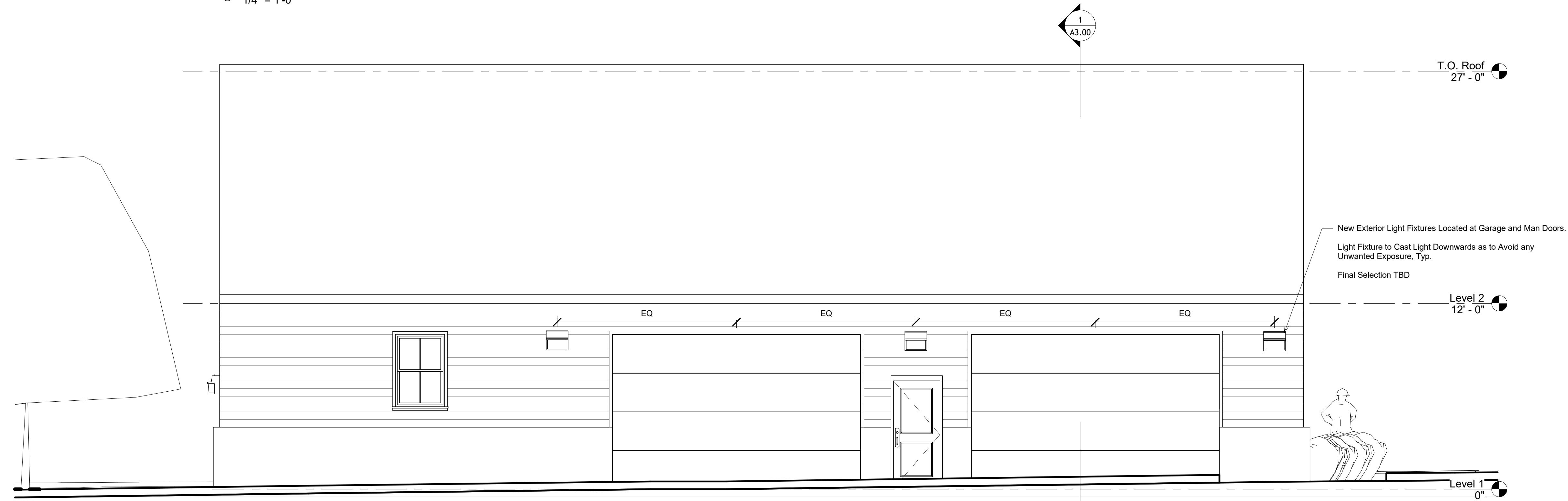
4 Exterior Elevation - West 1/4" = 1'-0"
