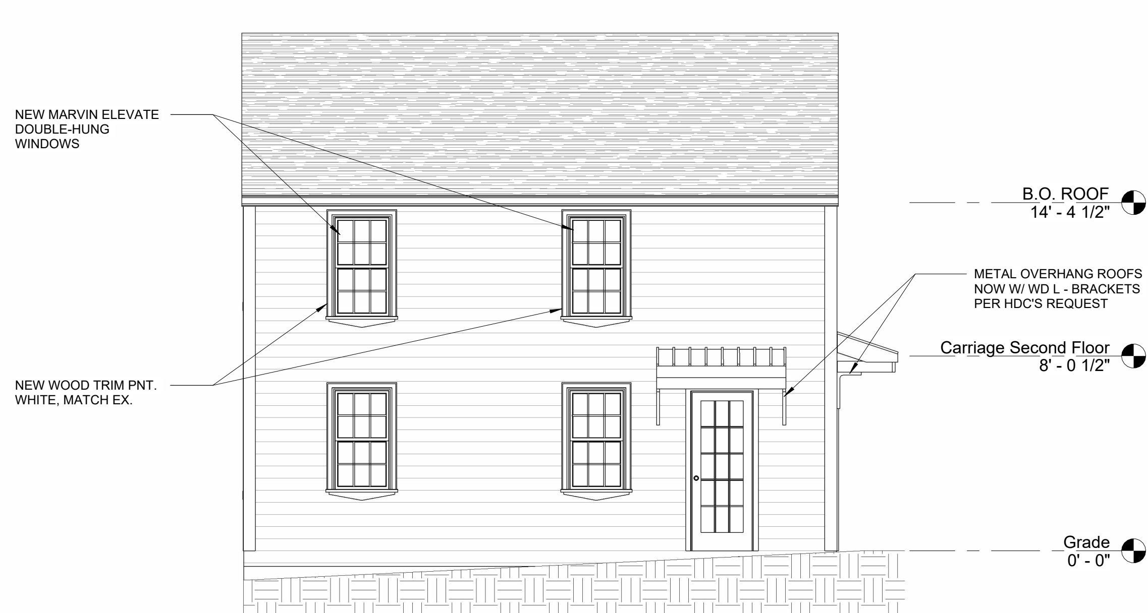
1 Proposed Carriage House South Elevation 1/4" = 1'-0"
