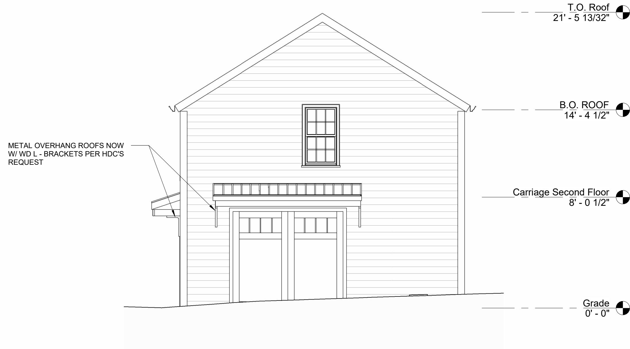
2 Proposed Carriage House East Elevation 1/4" = 1'-0"
