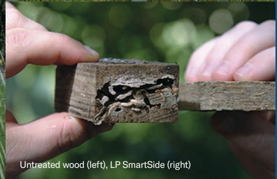
LP SmartSide product testing in Hilo, Hawaii
