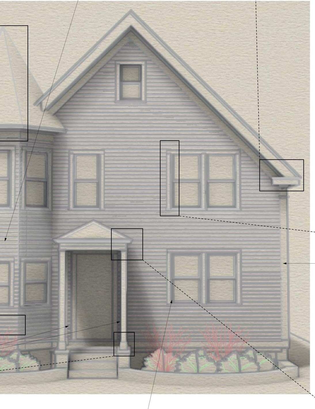
REPLACE CURRENT FIRST FLOOR LEVEL WINDOW - WITH SAME SIZE AS SECOND LEVEL WINDOW TO MEET BUILDING CODE/EGRESS REQUIREMENTS.
