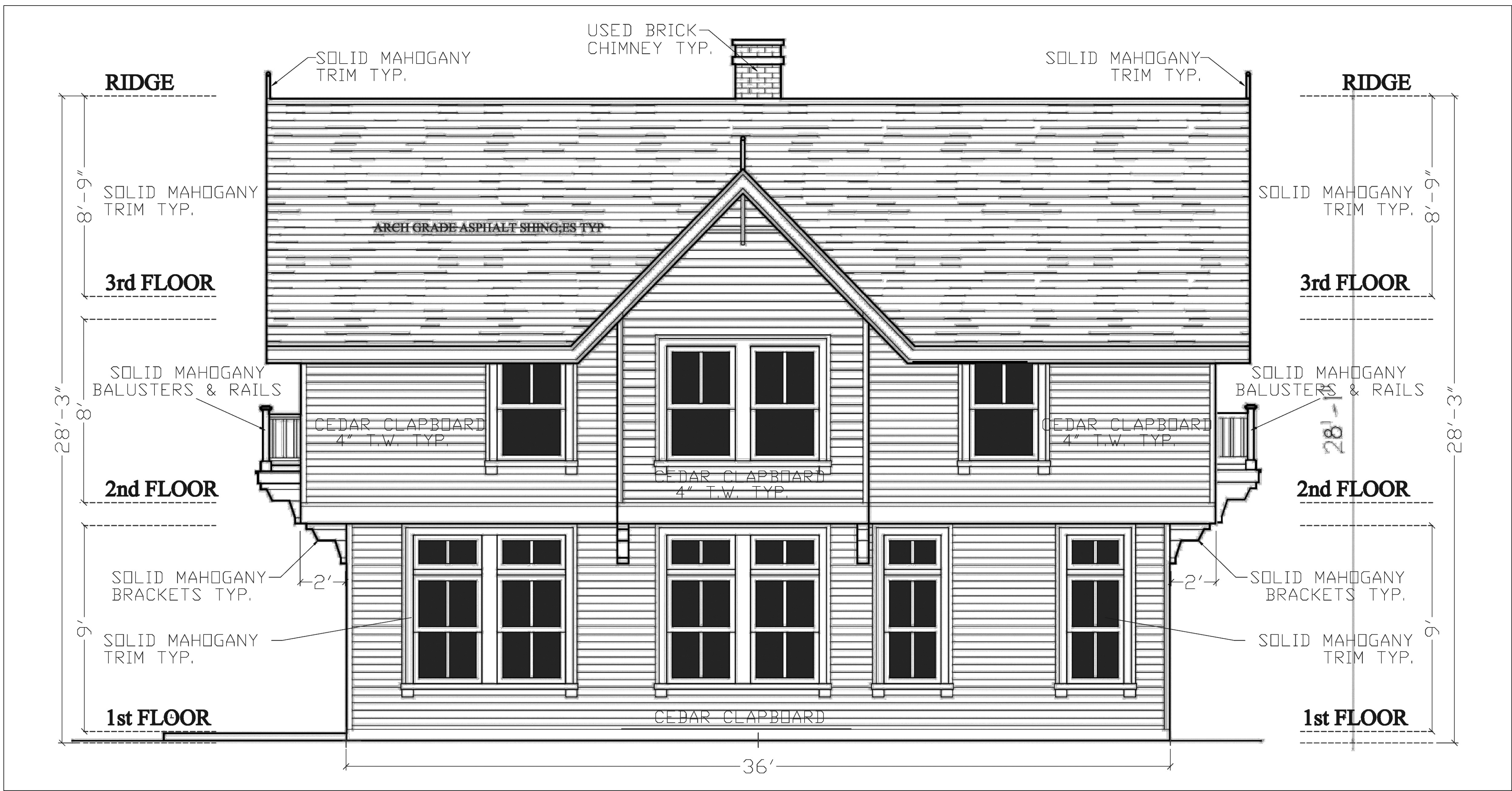
1 PREVIOUS TYPICAL SIDE ELEVATION - CARRIAGE HOUSE CLUSTER TYPE "A" 1200 HOPE STREET - BRISTOL - RHODE ISLAND SCALE: 1/4" = 1'-0"
