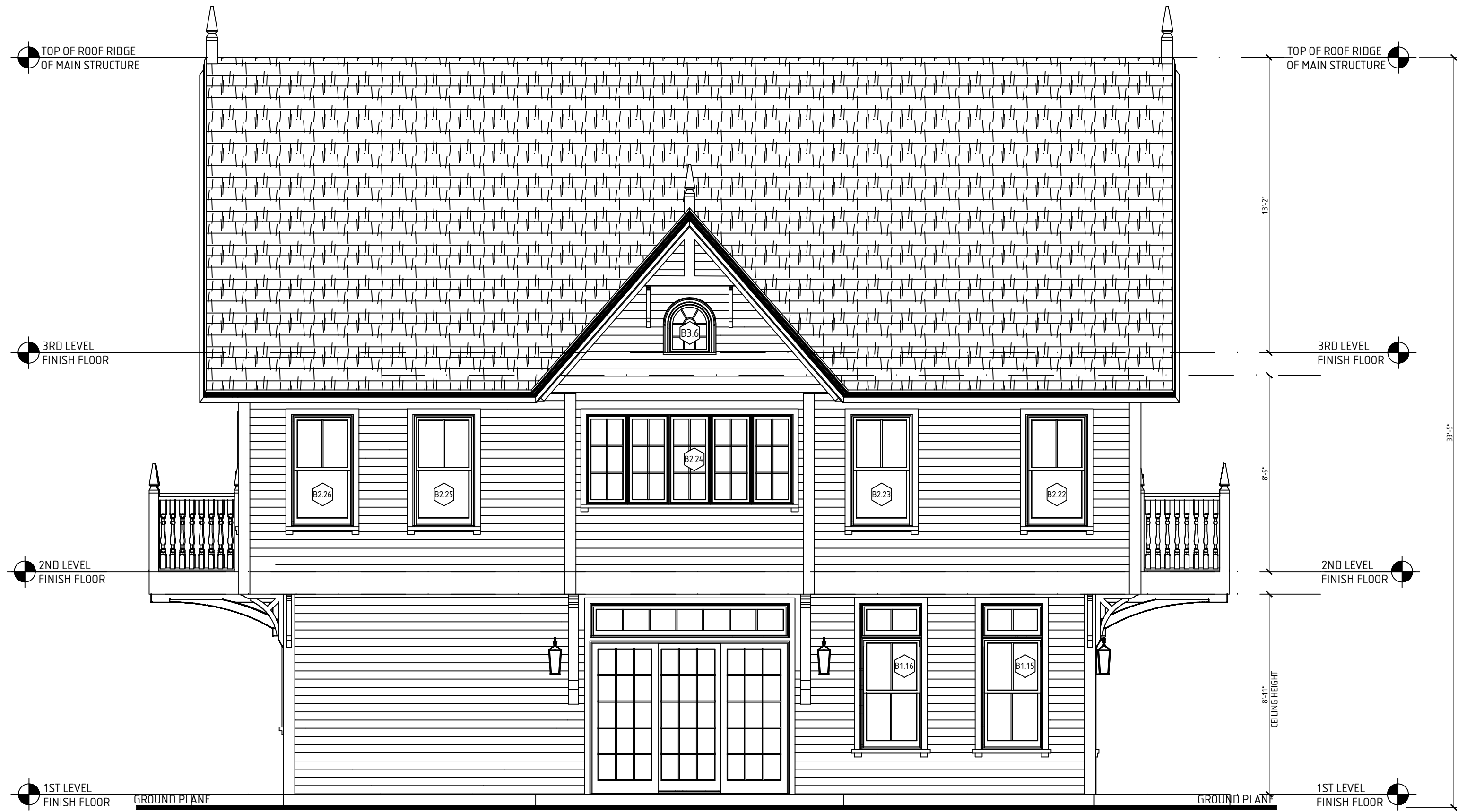
1 PROPOSED LEFT SIDE ELEVATION - CARRIAGE HOUSE CLUSTER TYPE "B" 1200 HOPE STREET - BRISTOL - RHODE ISLAND SCALE: 1/4" = 1'-0"
