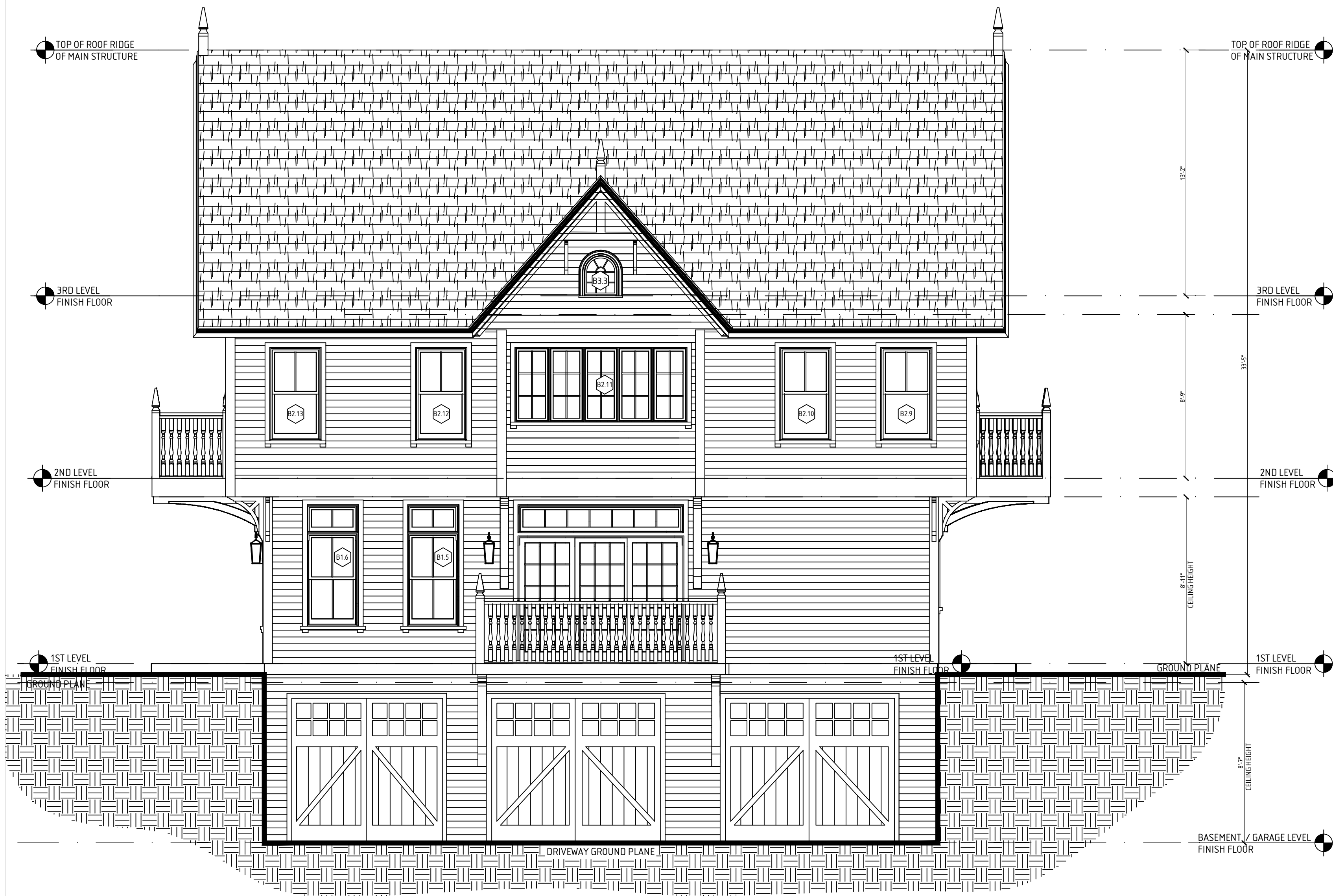
1 PROPOSED RIGHT SIDE ELEVATION - CARRIAGE HOUSE CLUSTER TYPE "B" 1200 HOPE STREET - BRISTOL - RHODE ISLAND SCALE: 1/4" = 1'-0"
