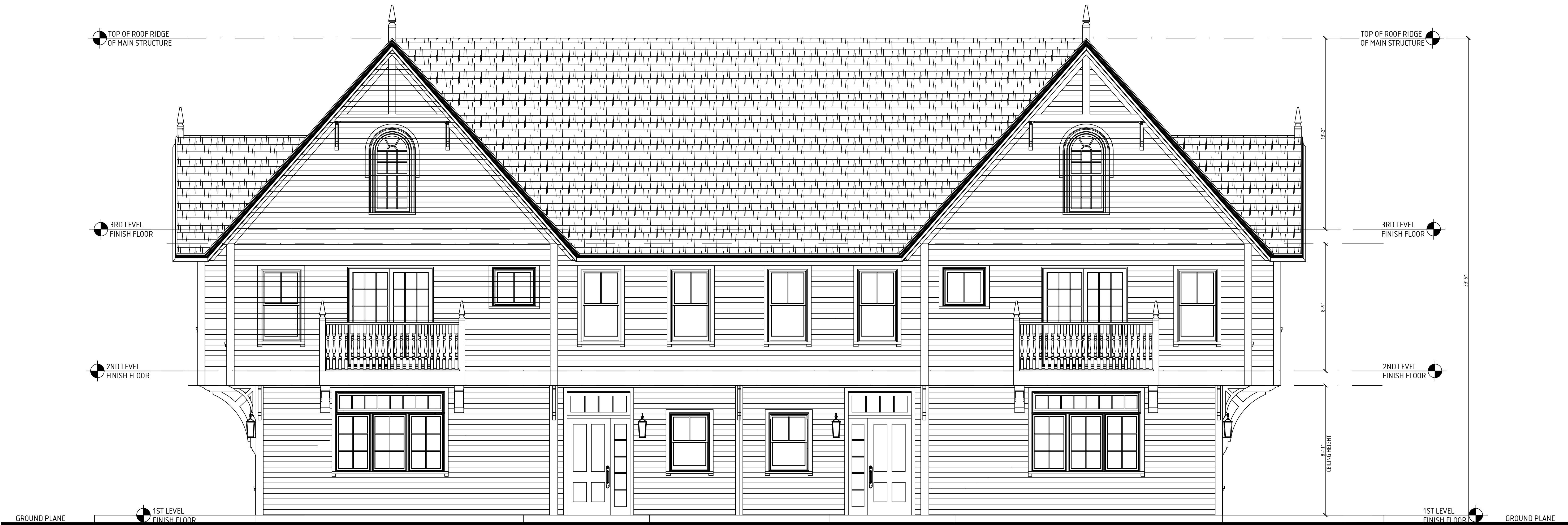
2 NEW TYPICAL BACK ELEVATION - CARRIAGE HOUSE CLUSTER TYPE "A" 1200 HOPE STREET - BRISTOL - RHODE ISLAND SCALE: 1/4" = 1'-0"
