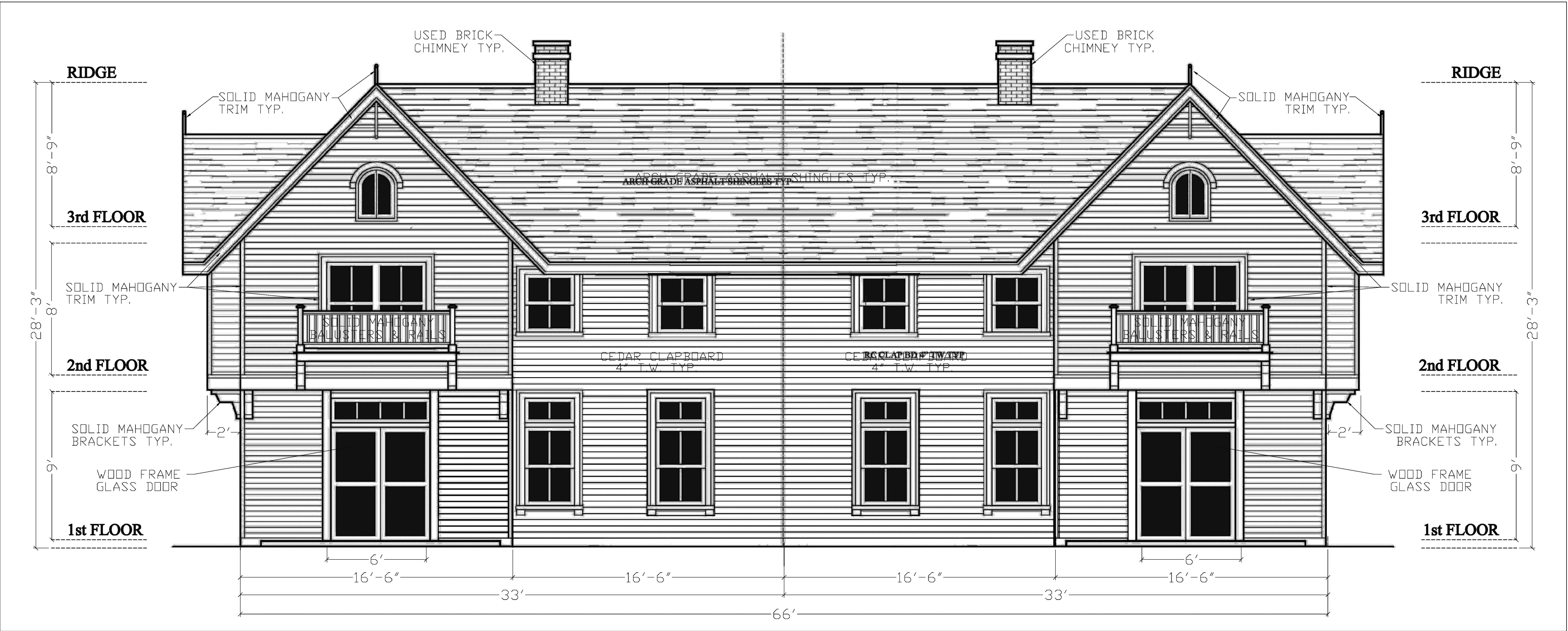
1 PREVIOUS TYPICAL BACK ELEVATION - CARRIAGE HOUSE CLUSTER TYPE "A" 1200 HOPE STREET - BRISTOL - RHODE ISLAND SCALE: 1/4" = 1'-0"
