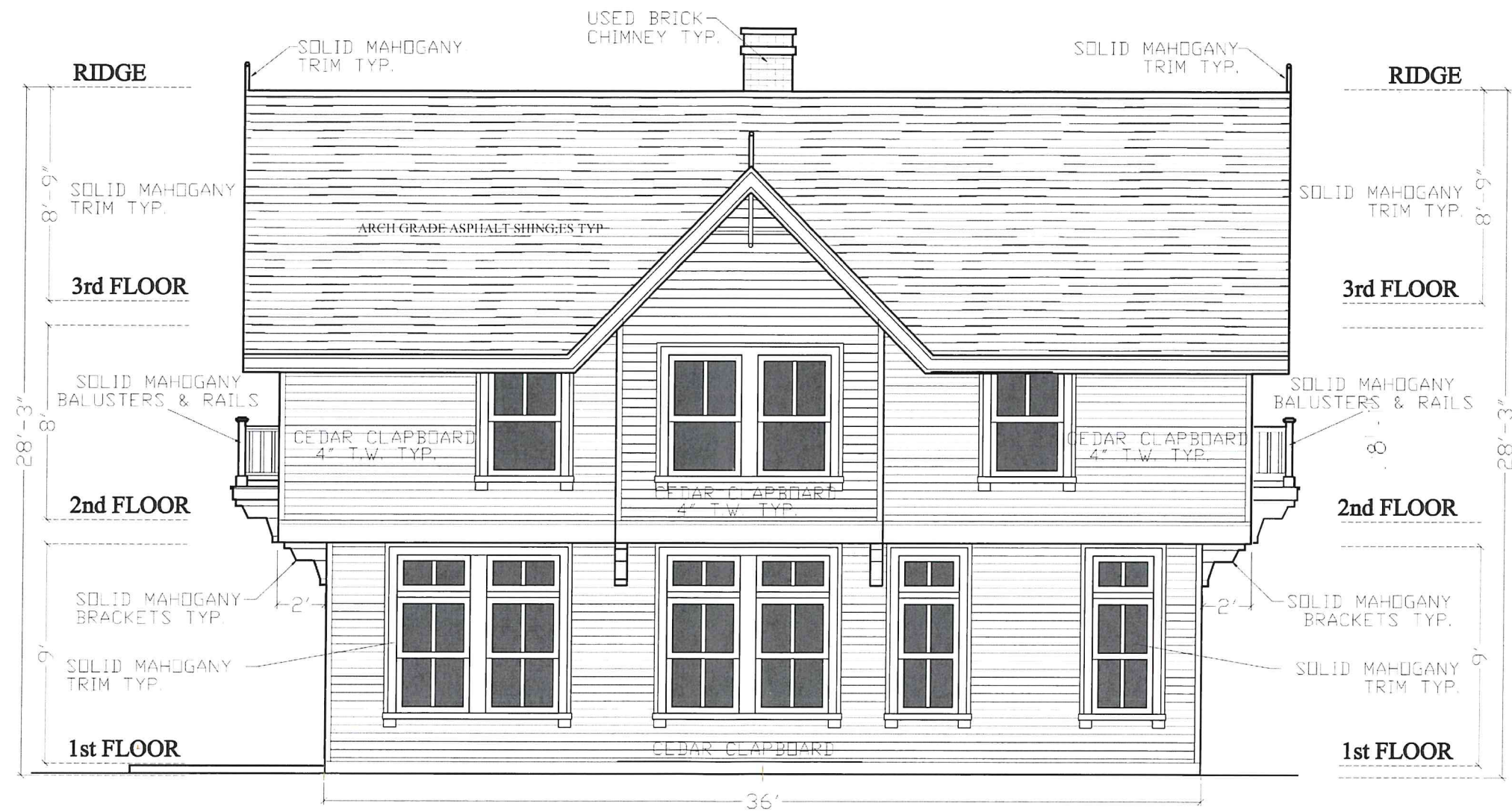
TYPICAL SIDE ELEVATION CARRIAGE HOUSE LONGFIELD ESTATES
