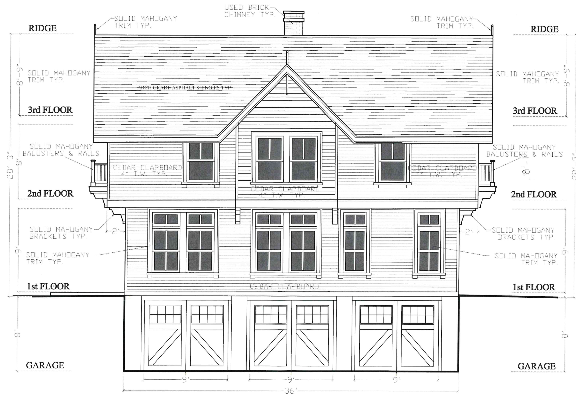
SIDE ELEVATION UNITS #1 & #2 CARRIAGE HOUSE LONGFIELD ESTATES
