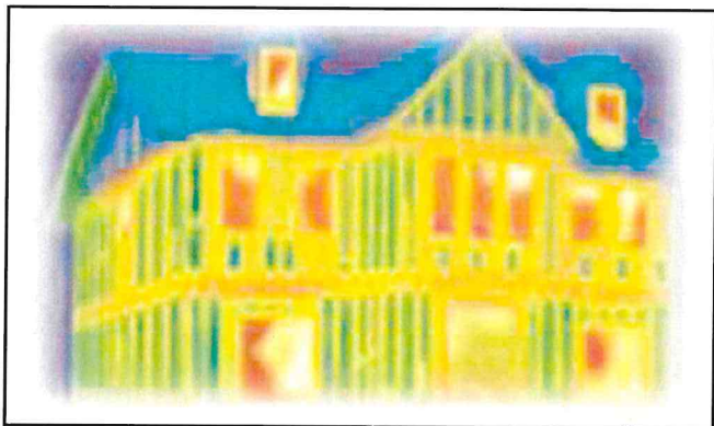
House with OSB and R-13 batts
