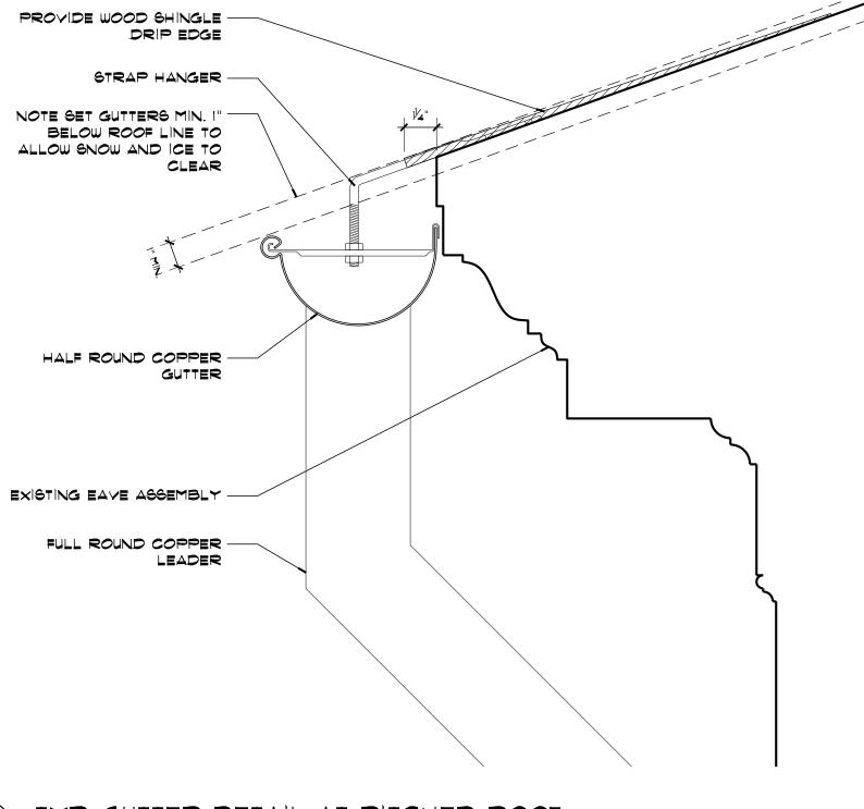
GUTTERS: 6" HALF ROUND 160Z HOO (COLD ROLLED) COPPER GUTTER IN 8' TO 10' LENGTHS. JOINT SEAMS TO BE LAPPED AND SOLDERED. END PIECES, MITERS AND OUTLETS TO BE PROVIDED.
