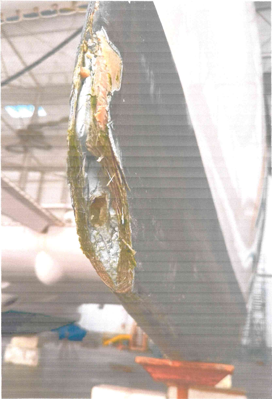
Damage at Bow – at and below waterline
