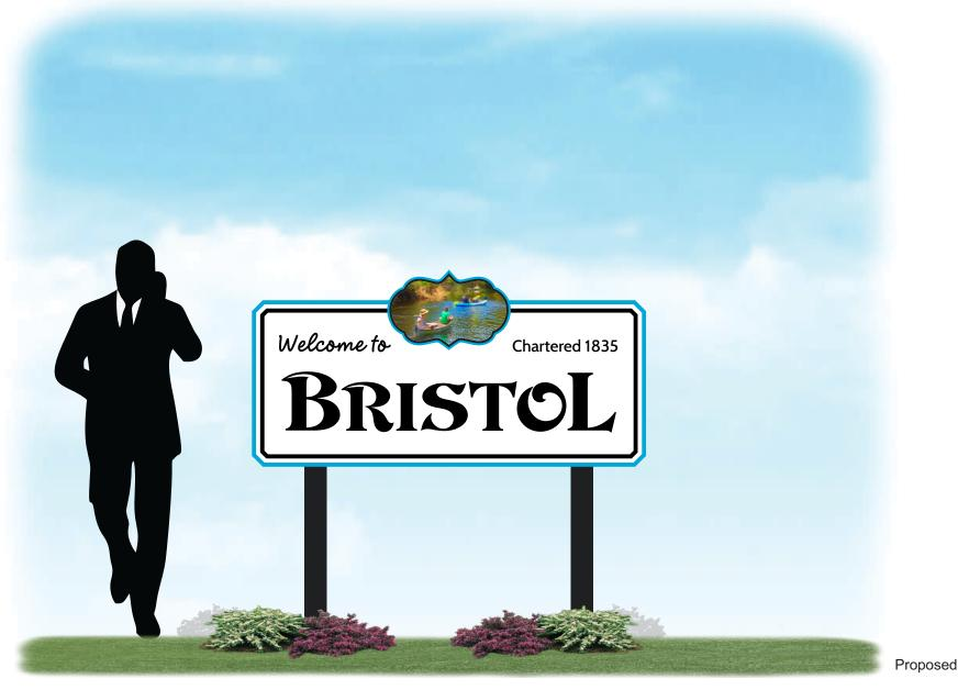
Four (4) Single Sided 35-1/2" tall x 71" wide x 2" non illuminated painted aluminum cloud cabinets. The cabinets have 1/4" flat cut out Black acrylic lettering and 1/4" flat cut out shape with printed graphic. All acrylic is mounted flush to the faces of the cabinets. Paint existing 4" sq wood posts Black and attached sign with 2" angle.
