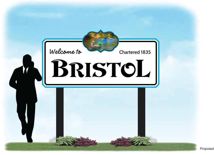
Four (4) Single Sided 47-1/2" tall x 95" wide x 2" non illuminated painted aluminum cloud cabinets. The cabinets have 1/4" flat cut out shape with printed graphic. All acrylic is mounted flush to the faces of the cabinets. Paint existing 6" sq wood posts Black and attach signs with 2" angle.
