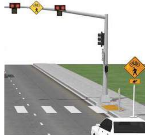
HAWK SIGNAL (High-Intensity Activated crossWalk)
