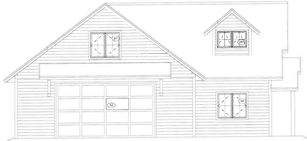
1 FRONT ELEVATION A2.1 1/4" = 1'-0"
