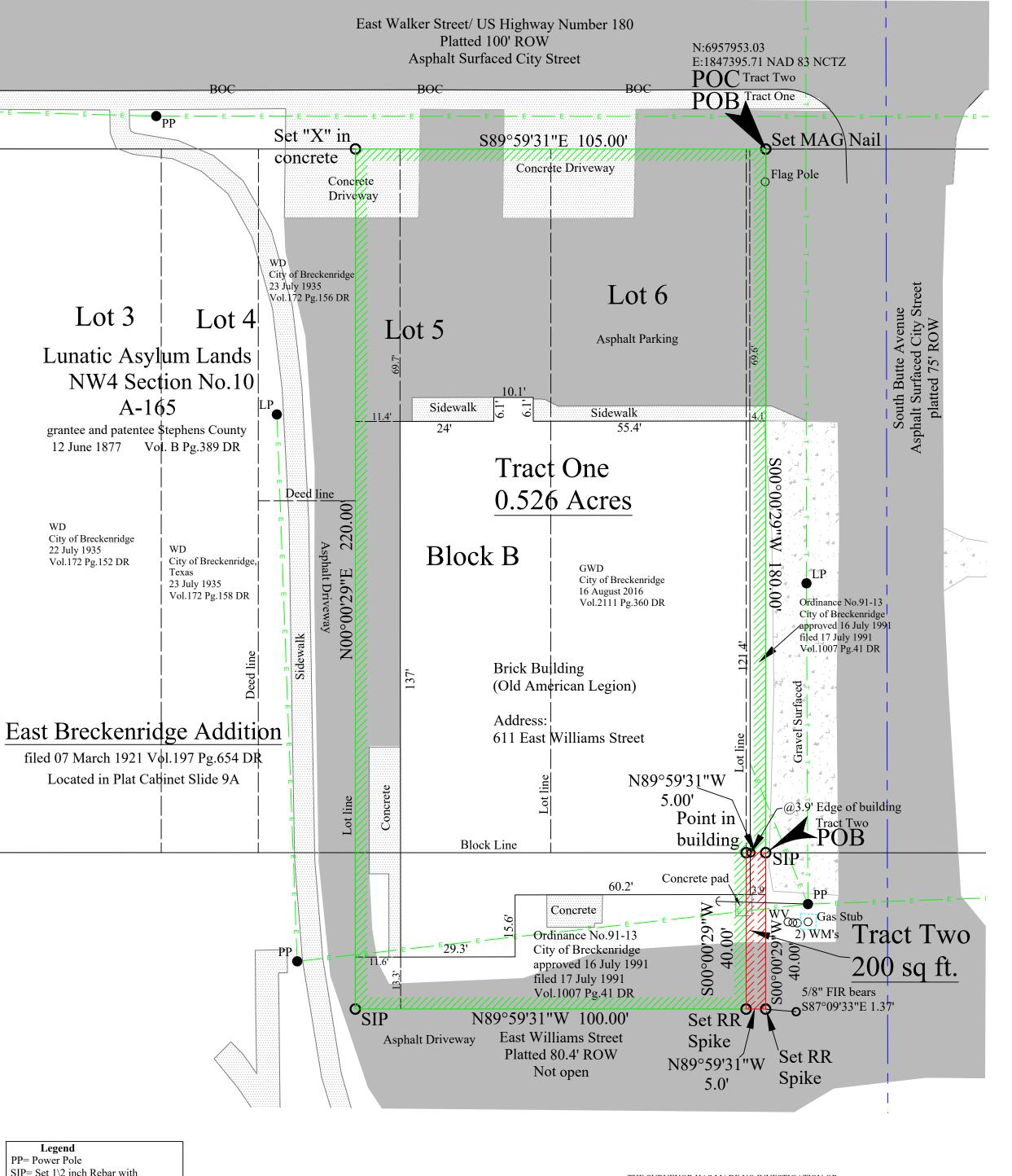
SIP= Set 1\2 inch Rebar with plastic cap marked OWEN SURV 5560
