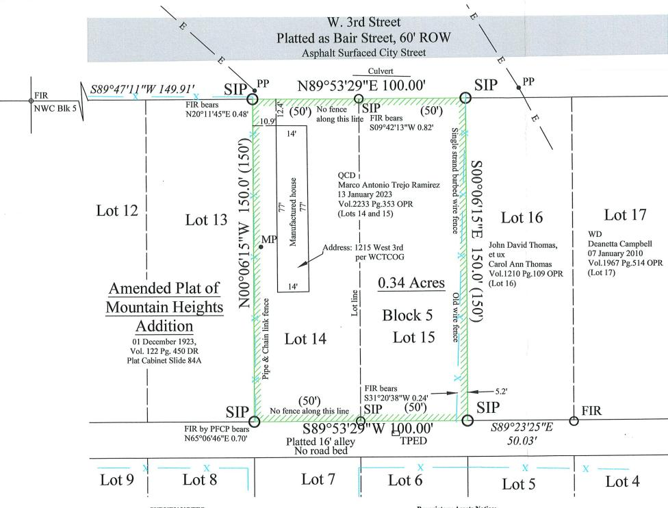
Legend SIP= Set 1\2 inch Rebar with plastic cap marked **OWEN SURV 5560**
