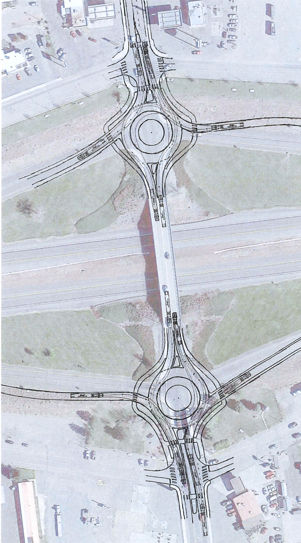
Figure 8 – Refined Circulation Alternative #2 Sketch-Level Layout (with WB-67 Truck Turning Template)
