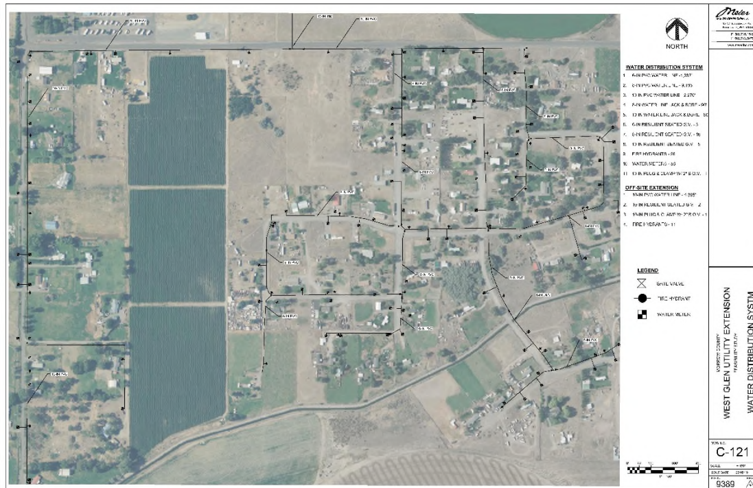
Figure 1: Preliminary Water Distribution System Layout
