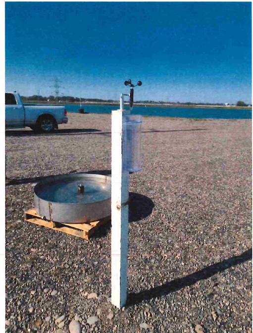
Photo 1: Leak test equipment setup.
