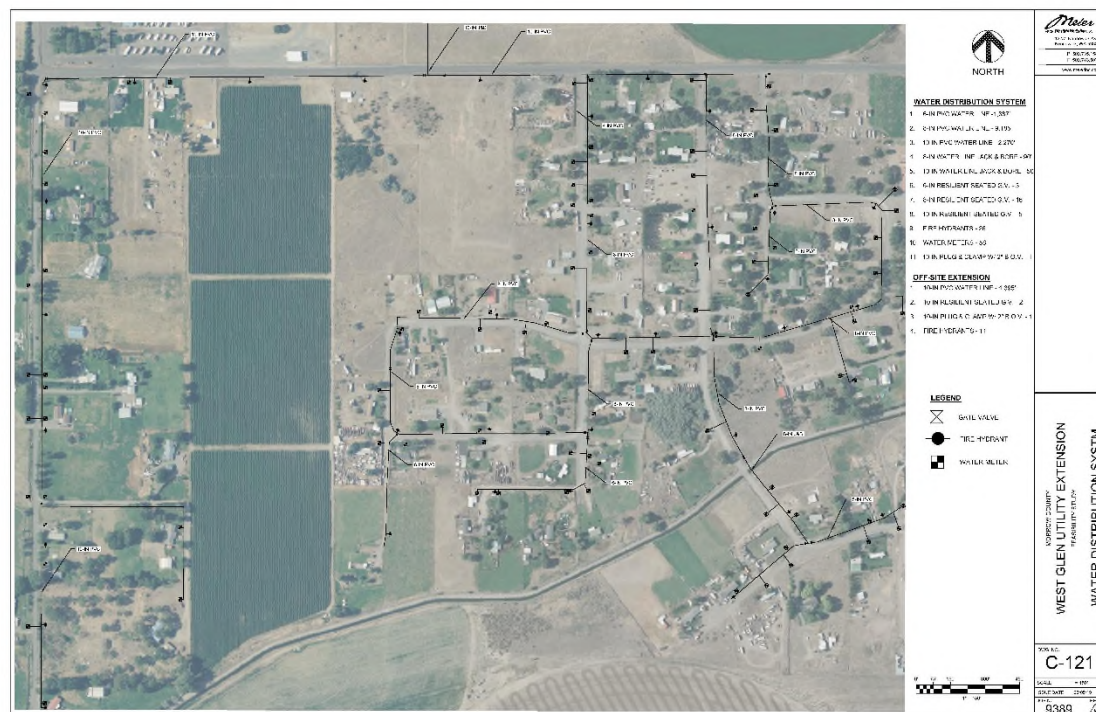
Figure 1: Preliminary Water Distribution System Layout
