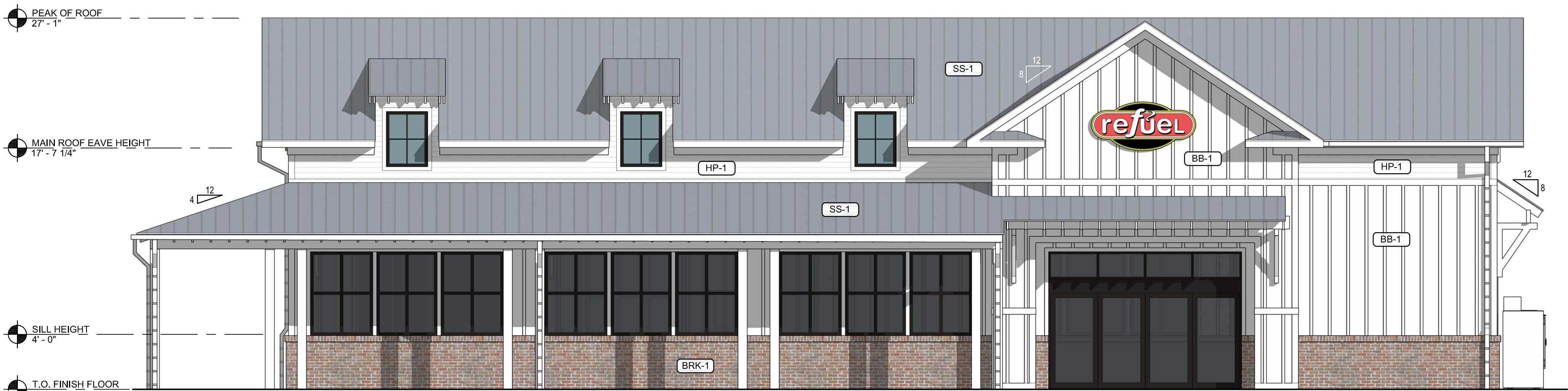
1 ELEVATION - FRONT (NORTH FACE - SC HIGHWAY 46) 3/16" = 1'-0"
