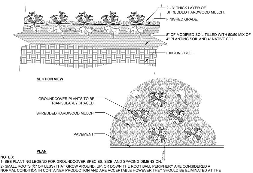
1- SEE PLANTING LEGEND FOR GROUNDCOVER SPECIES, SIZE, AND SPACING DIMENSION. 2- SMALL ROOTS (¼" OR LESS) THAT GROW AROUND, UP, OR DOWN THE ROOT BALL PERIPHERY ARE CONSIDERED A NORMAL CONDITION IN CONTAINER PRODUCTION AND ARE ACCEPTABLE HOWEVER THEY SHOULD BE ELIMINATED AT THE TIME OF PLANTING. ROOTS ON THE PERIPERHY CAN BE REMOVED AT THE TIME OF PLANTING. (SEE ROOT BALL SHAVING CONTAINER DETAIL). 3- SETTLE SOIL AROUND ROOT BALL OF EACH GROUNDCOVER PRIOR TO MULCHING.
