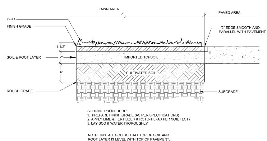
SOD INSTALLATION URBAN TREE FOUNDATION © 2014 OPEN SOURCE FREE TO USE NOT TO SCALE 0002-01
