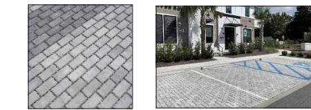
Model: Hydrashed Classic Brick Style Permeable Pavers - 60mm Finish: Tabby Color: Battery Gray Pattern: Running Bond Size: 7 7/8" x 3 7/8"
