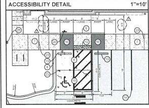
NEW FIVE PERVIOUS PAVERS PARKING SPACES SEE DETAILS SHEET C05.02
