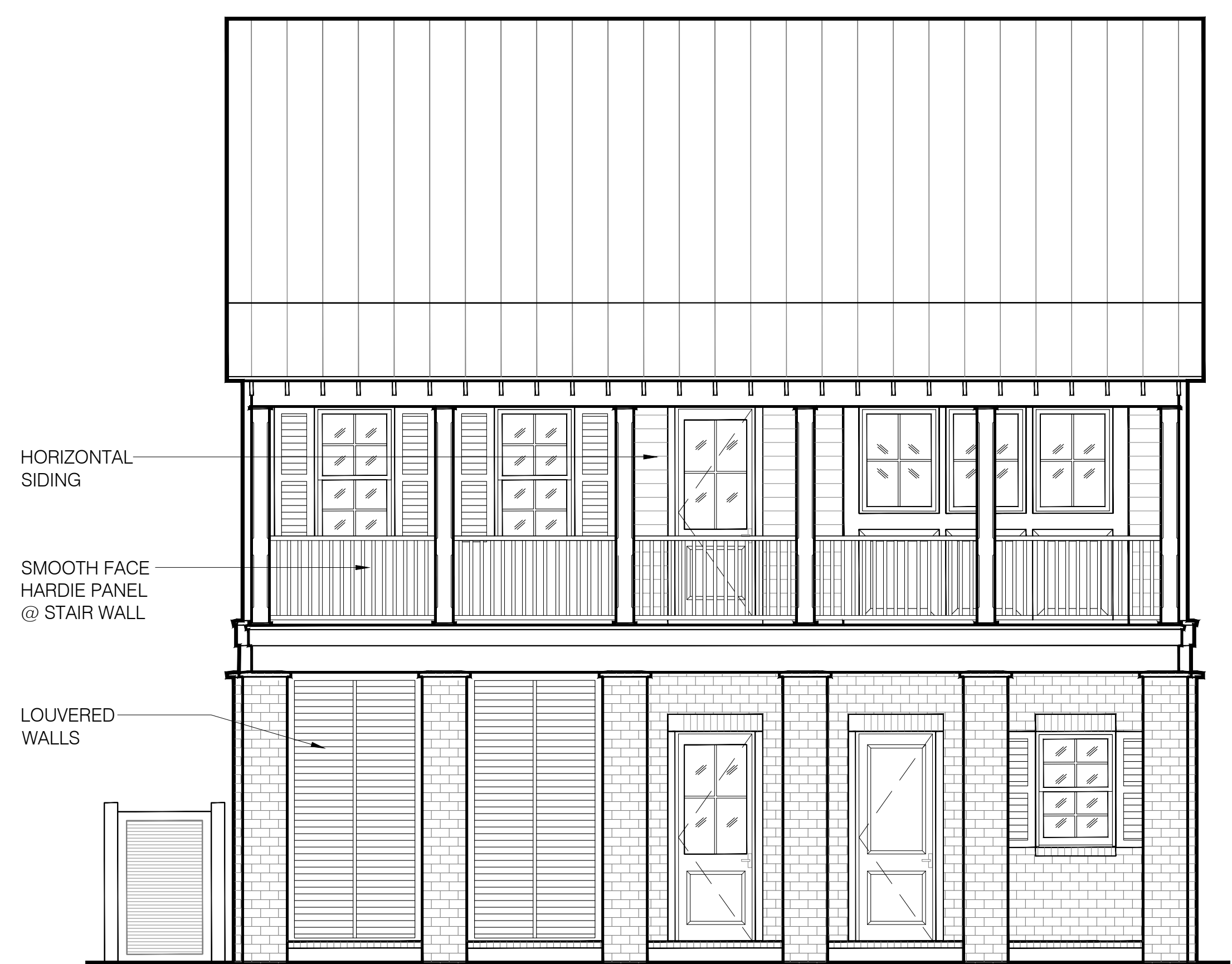
C REAR ELEVATION @ MAIN BLDG. A5 SCALE: 1/4"=1'-0"
