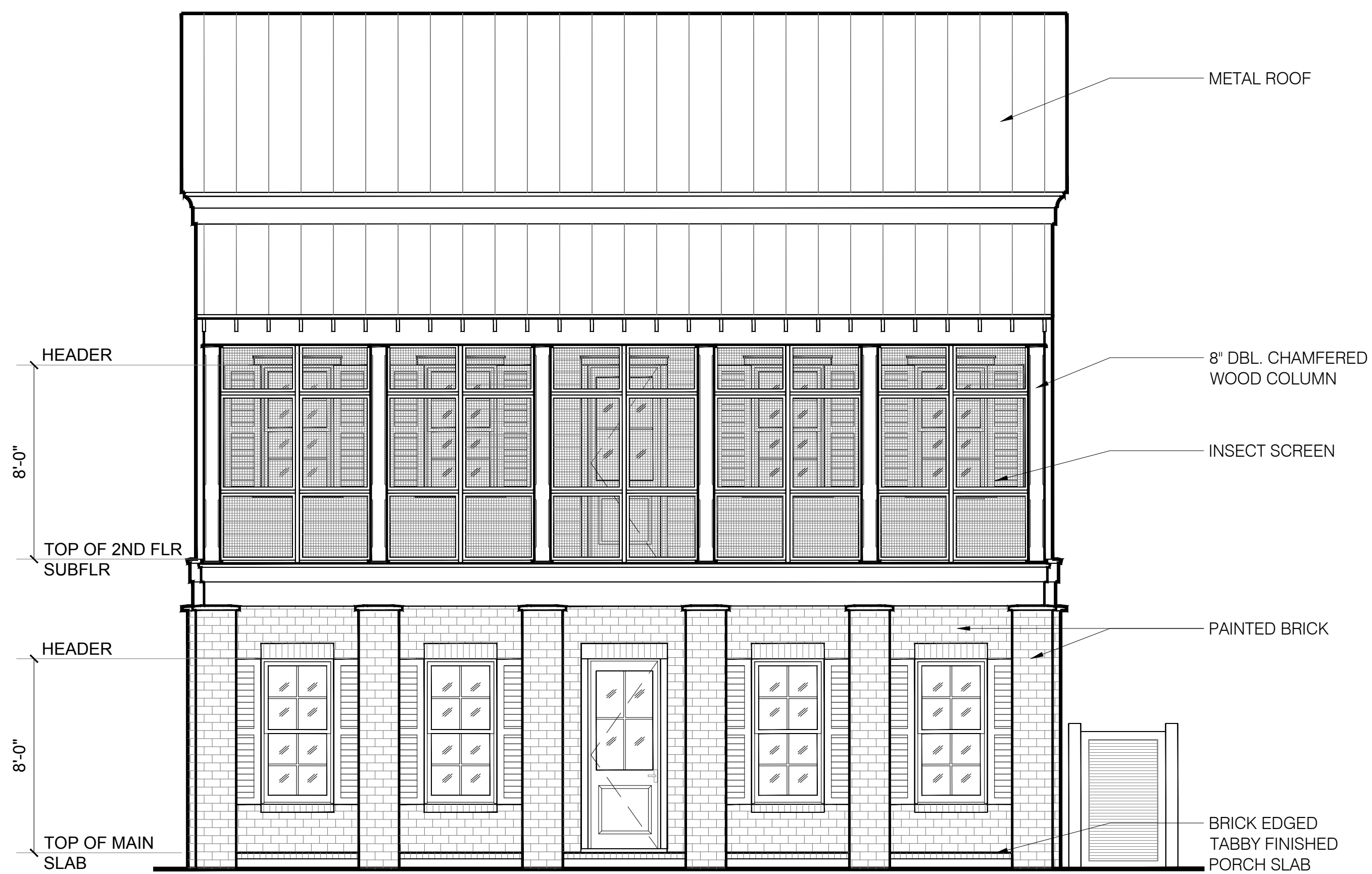
A FRONT ELEVATION @ MAIN BLDG. A5 SCALE: 1/4"=1'-0"
