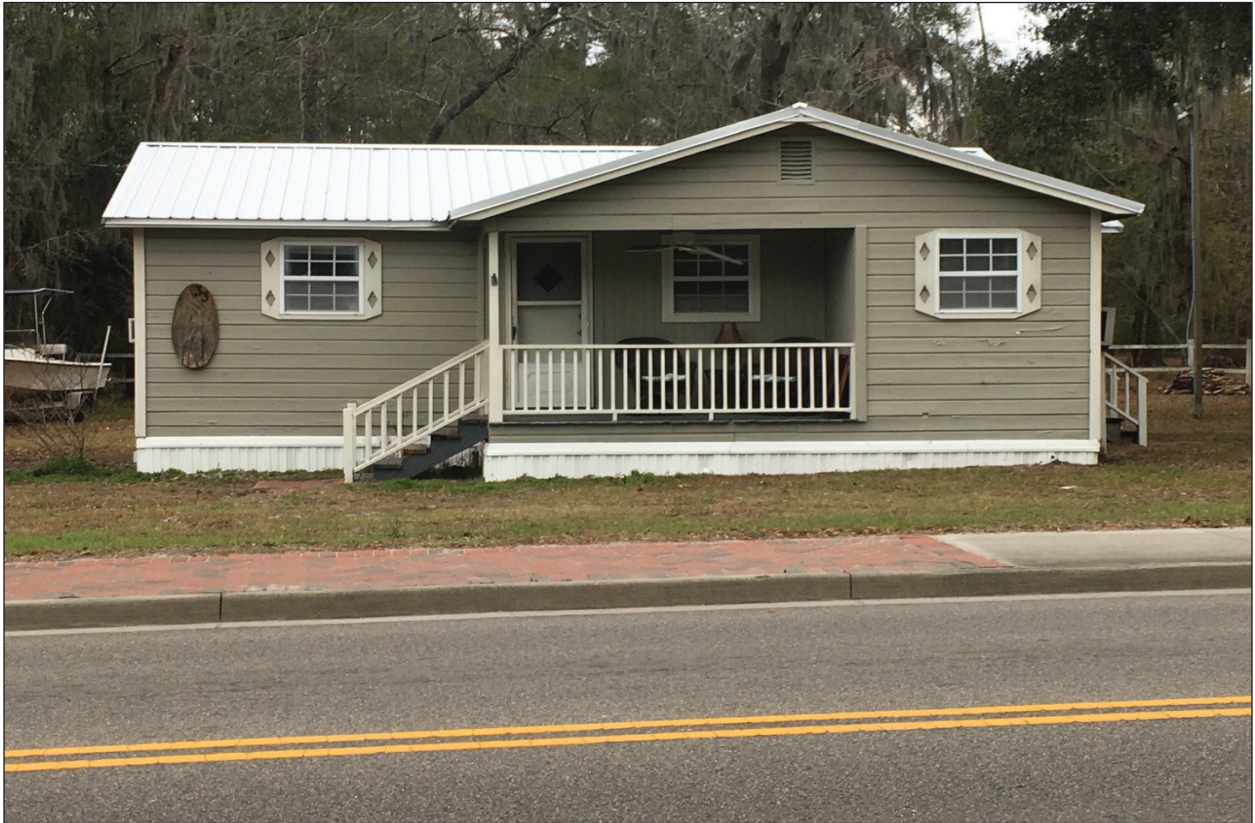
Figure 4.16 Example of a Minimal Traditional house within the Bluffton Historic District Survey Area featuring a projecting gable porch (Resource 5322, 33 Bruin Road).
