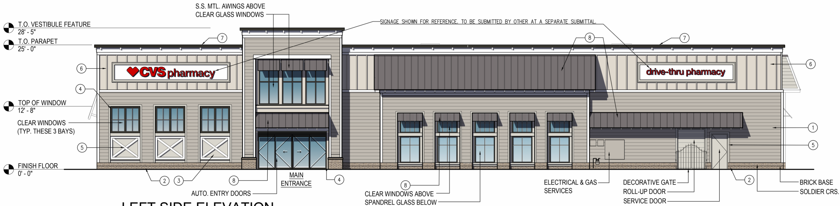
LEFT SIDE ELEVATION
