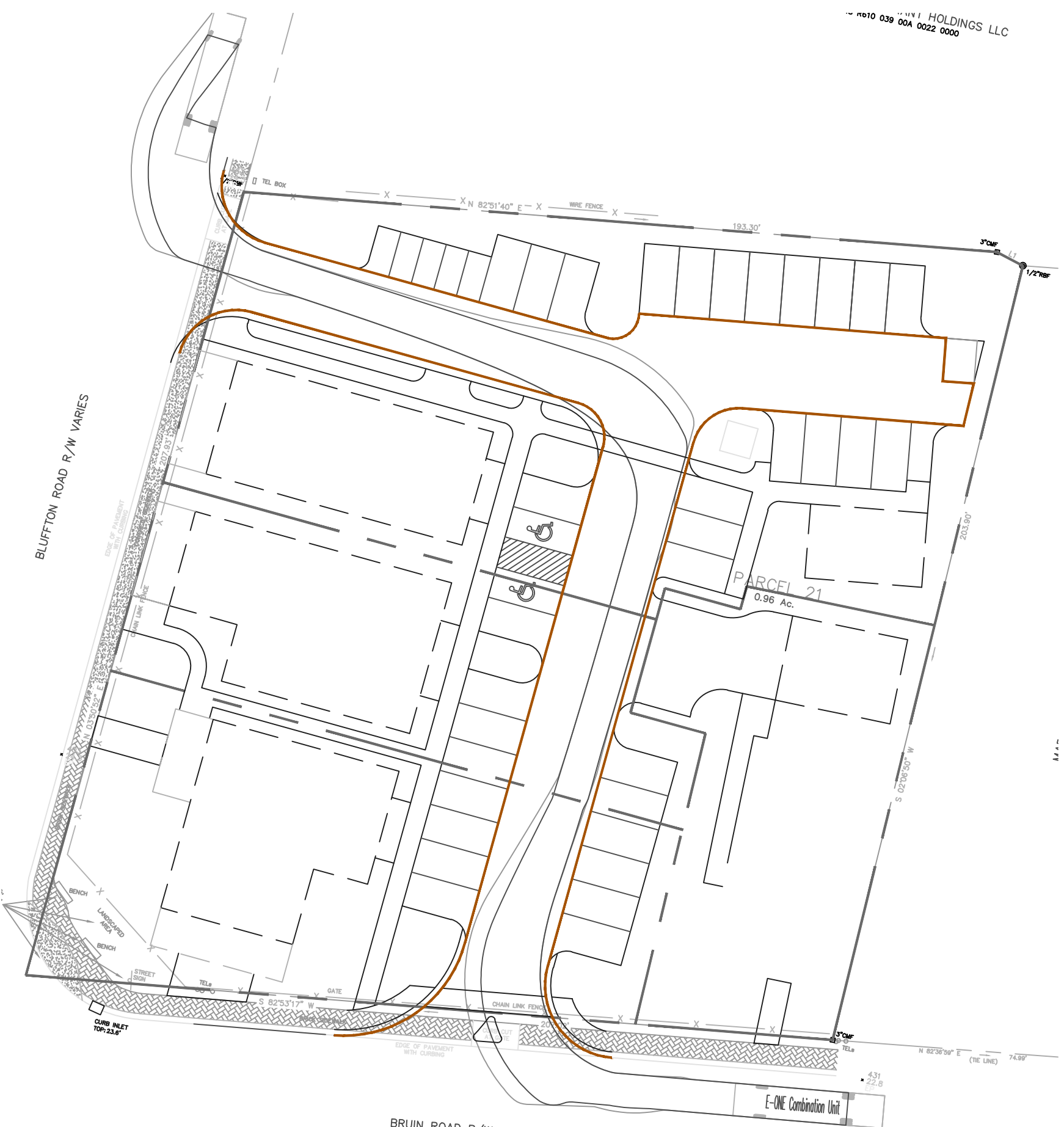
DESIGN VEHICLE FIRE TRUCK - E-ONE CYCLONE 11 CHASSIS WIDTH = 8.33' LENGTH = 46.33' W/W RADIUS = 44.27'
