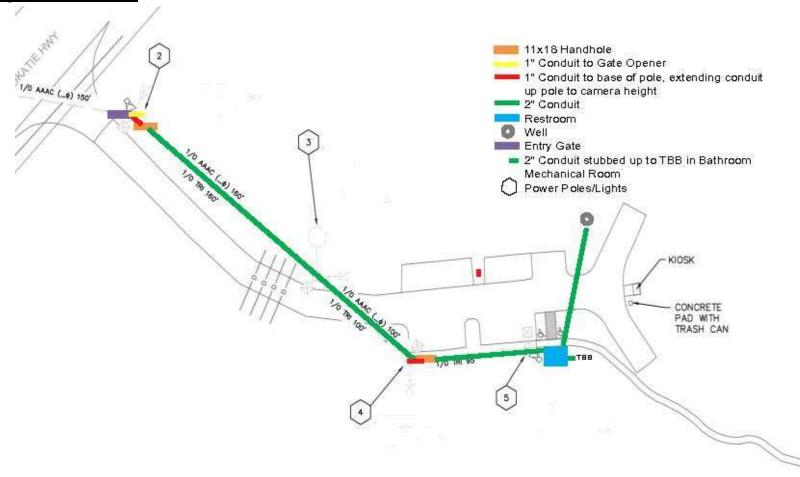
The interwoven scope of connections include the conduit and electrical work for the restroom, well, security cameras and electronic gate which all run to the TBB (telephone backboard) in the utility room of the restroom.
